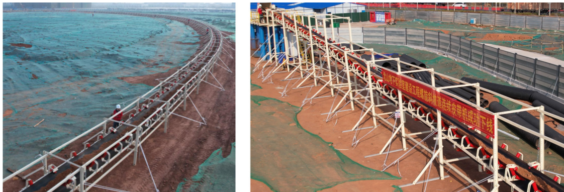
Fig. 6 Specialized conveyor system for muck transportation in factory test.
