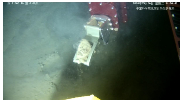
Fig. 3 Underwater manipulator grabbing of Haidou-1 at depths exceeding 10000 meters.
