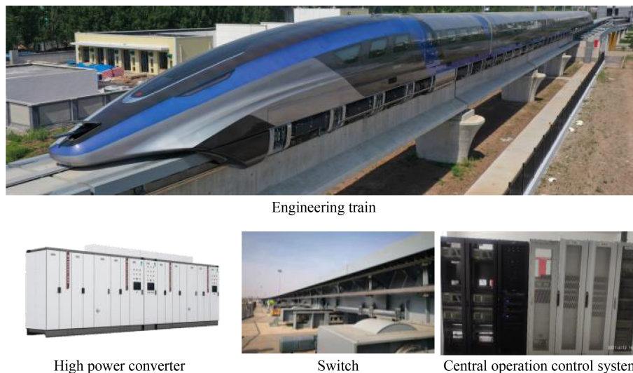
Fig. 3 Whole system engineering prototype.
