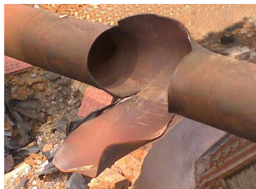
Fig. 1 Full-scale pipeline blasting test.
