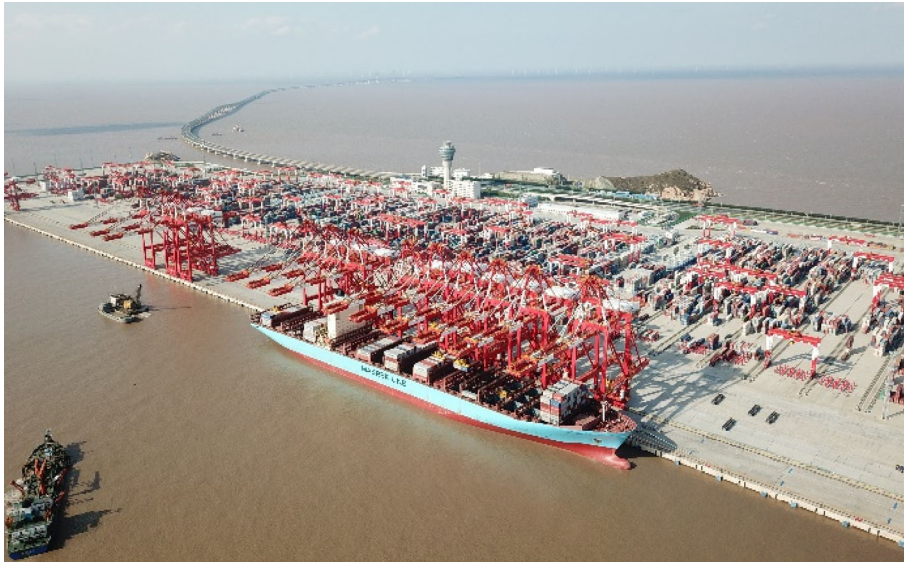
Fig. 8 Nine AQC's work together to handle a trip-E ultra-large ship.
