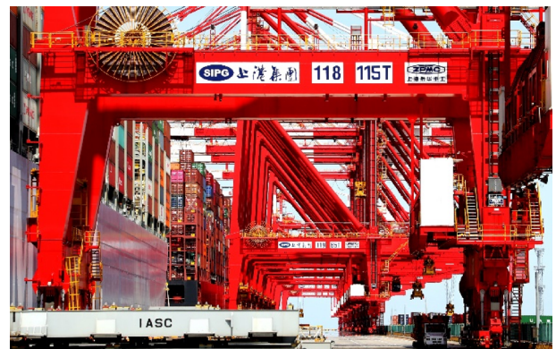
Fig. 4 Remotely controlled automated quay cranes (RC-AQCs).
