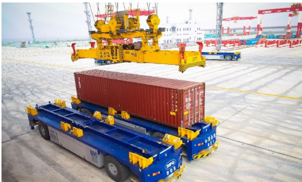
Fig. 6 AGVs using automatically-replaced batteries which supports automated lifting.
