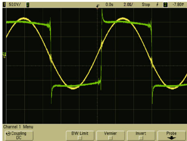
Fig. 18 CH1: resonant voltage [volt scale: 40 V/div]. CH2: resonant current [ampere scale: 0.5 A/div] for LCL-T SPRC
