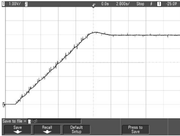
Fig. 17 Experimental graph of speed variation for the step change in reference speed using the conventional PID controller
