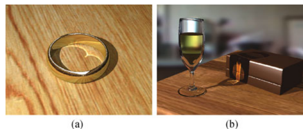
Fig. 18 Caustics rendering using photon mapping [3]. (a) A metal ring; (b) a glass of champagne
