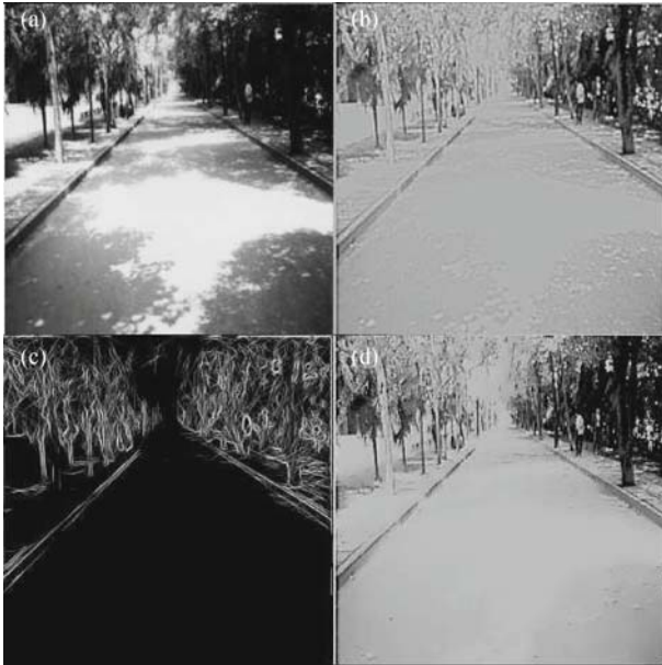
Fig. 18 FACADE processing of roadside scenery images. (a) Input image; (b) output of the LGN; (c) summed BCS output; (d) output after the FCS filling-in
