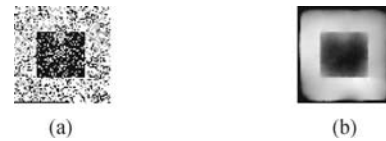
Fig. 8 (a) The test image containing a square object in a noisy background, where the integrity of the boundary contour of the square is disrupted by the strong noise; (b) the filling-in output of the FACADE-based image processing application in this paper with typical model parameters. The FACADE approach smooths the strong noise while at the same time preserving the clarity of the object boundary and fixes the broken contour of the square object automatically, thus making it easier for further object recognition approaches to generate a reasonable image segmentation and separate the square object from the rather noisy background
