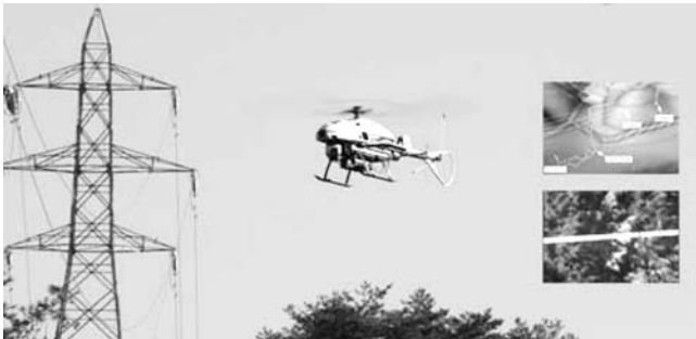
Fig. 14 Sky Surveyor inspecting power transmission line
