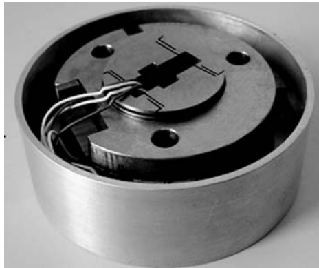
Fig. 8 Inner structure of PZT motor
