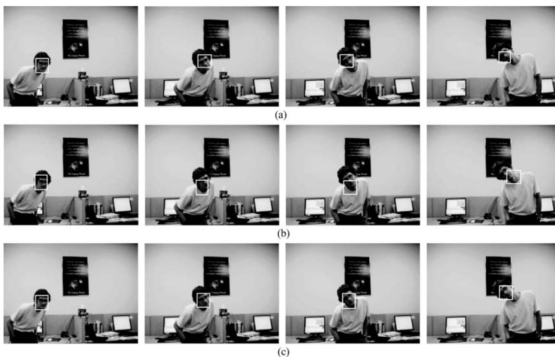
Fig. 3 Tracking a face with different poses. (a) Intensity cue; (b) edge cue; (c) our method (From left to right they are frames 343, 387, 402 and 435)
