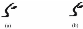
Fig. 3 Disjointed "5" detected and merged (a) Example of a "5" with a disjointed top stroke; (b) Disjointed top stroke merged
