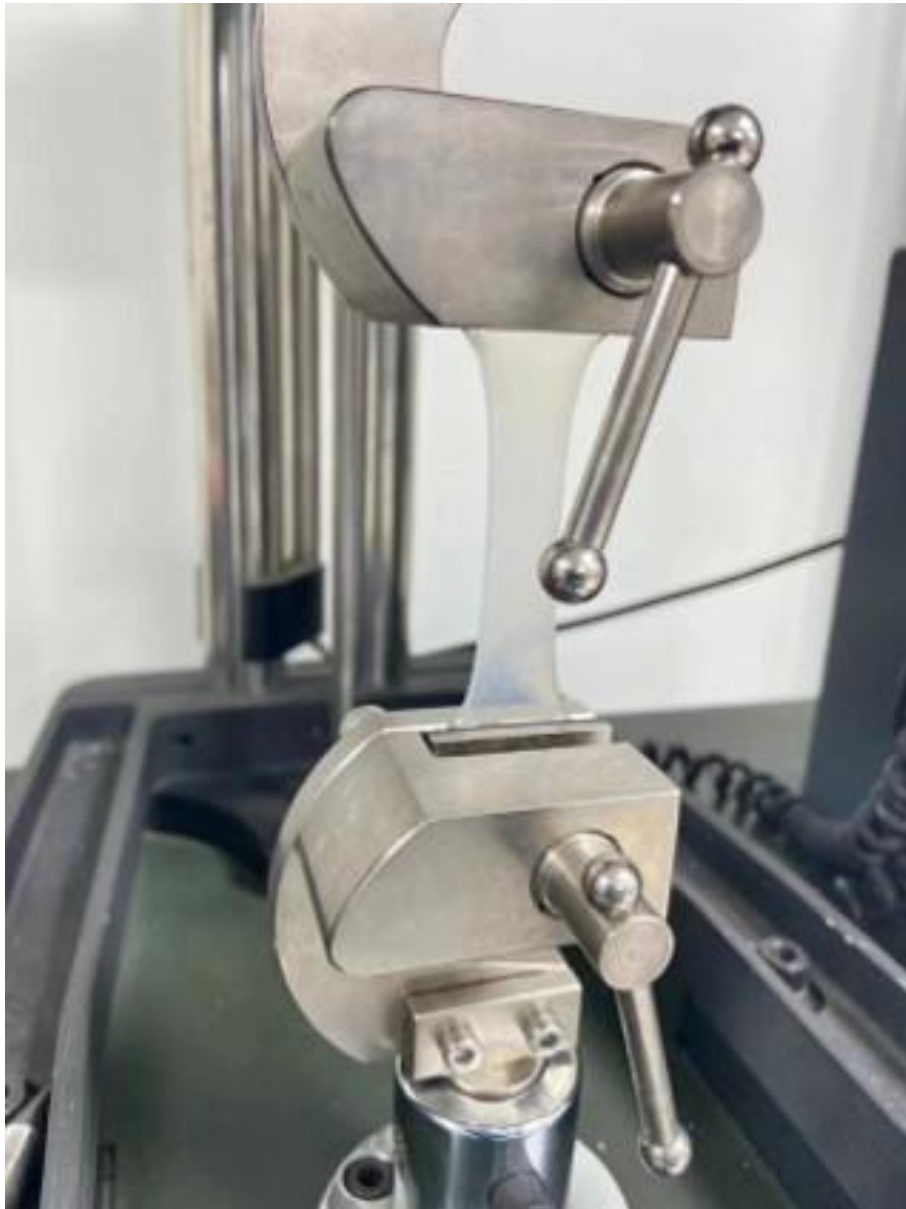
Fig. S8. Optical photograph of the stretched PANa-PVP-TiO 2 (NH 2 ) GPE.
