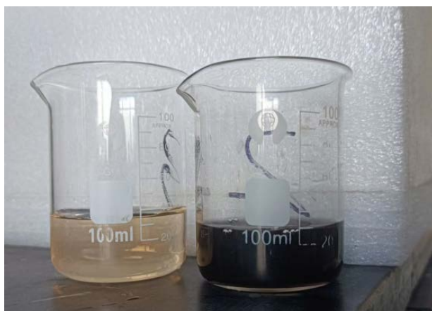
Figure. S5 The effluent upon addition of potassium iodide and indicator at the space time of 96.41 \text{g}_{\text{zeolite}} \cdot \text{h} / \text{mol}_{\text{phenol}} (left) and 61.95 \text{g}_{\text{zeolite}} \cdot \text{h} / \text{mol}_{\text{phenol}} (right)
