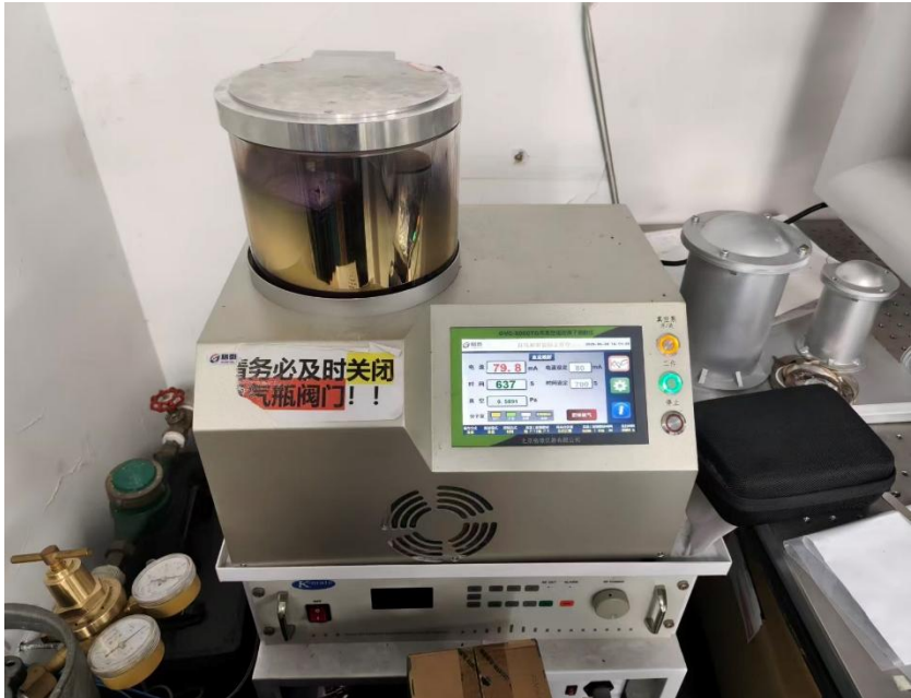
Fig. S4. Magnetron sputtering system for Pt electrode fabrication.
