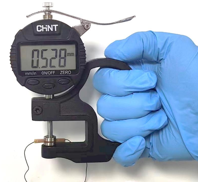
Fig. S6. Thickness measurement of the assembled flexible pressure sensor.
