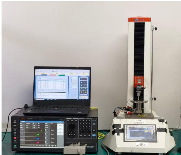
Fig. S7. Pressure calibration setup for sensor characterization.
