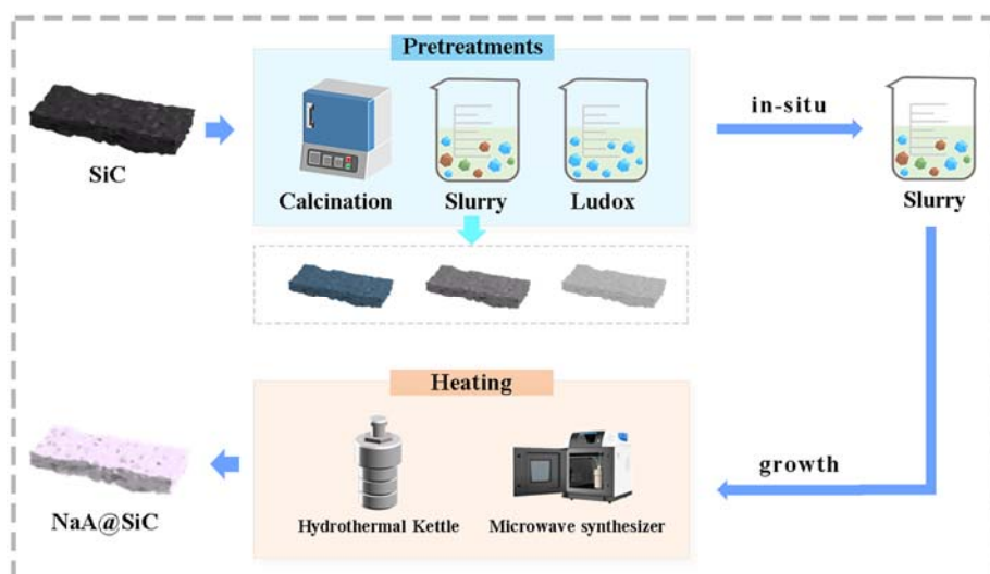
Fig.S1 Schematic illustration of the synthesis process for preparing NaA@SiC.
