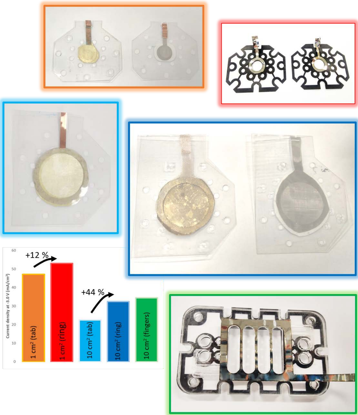
Figure S6 – Current collectors and their impact on current density for 1 and 10 cm 2 electrode area
