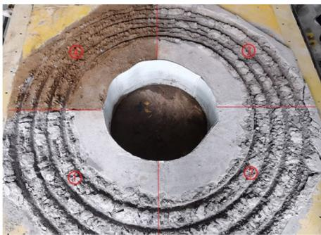
Fig. 2 Excavation face model in soft-hard varied strata.
