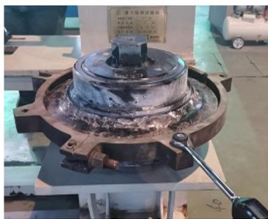
**Fig. 13** Starting torque measurement of the disc cutter.
