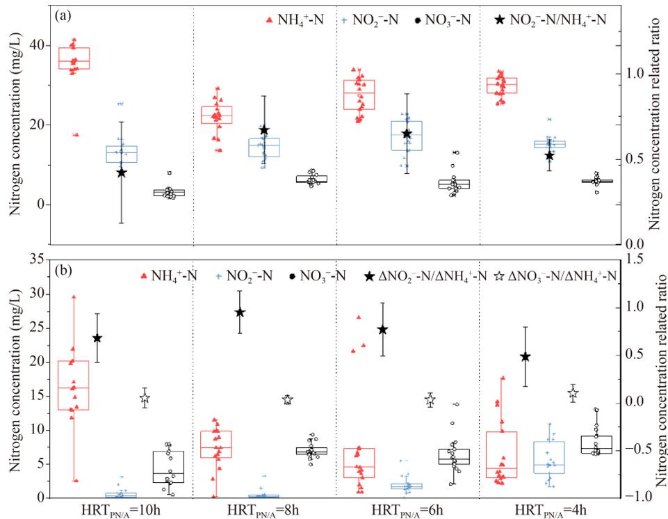
**Fig. 2** (a) Nitrogen concentrations and the  $\text{NO}_2^-$ -N/ $\text{NH}_4^+$ -N value of the PN-SBR effluent at various HRTs; (b) nitrogen concentrations,  $\Delta\text{NO}_2^-$ -N/ $\Delta\text{NH}_4^+$ -N, and  $\Delta\text{NO}_3^-$ -N/ $\Delta\text{NH}_4^+$ -N of the Anammox-UASB at various HRTs.
