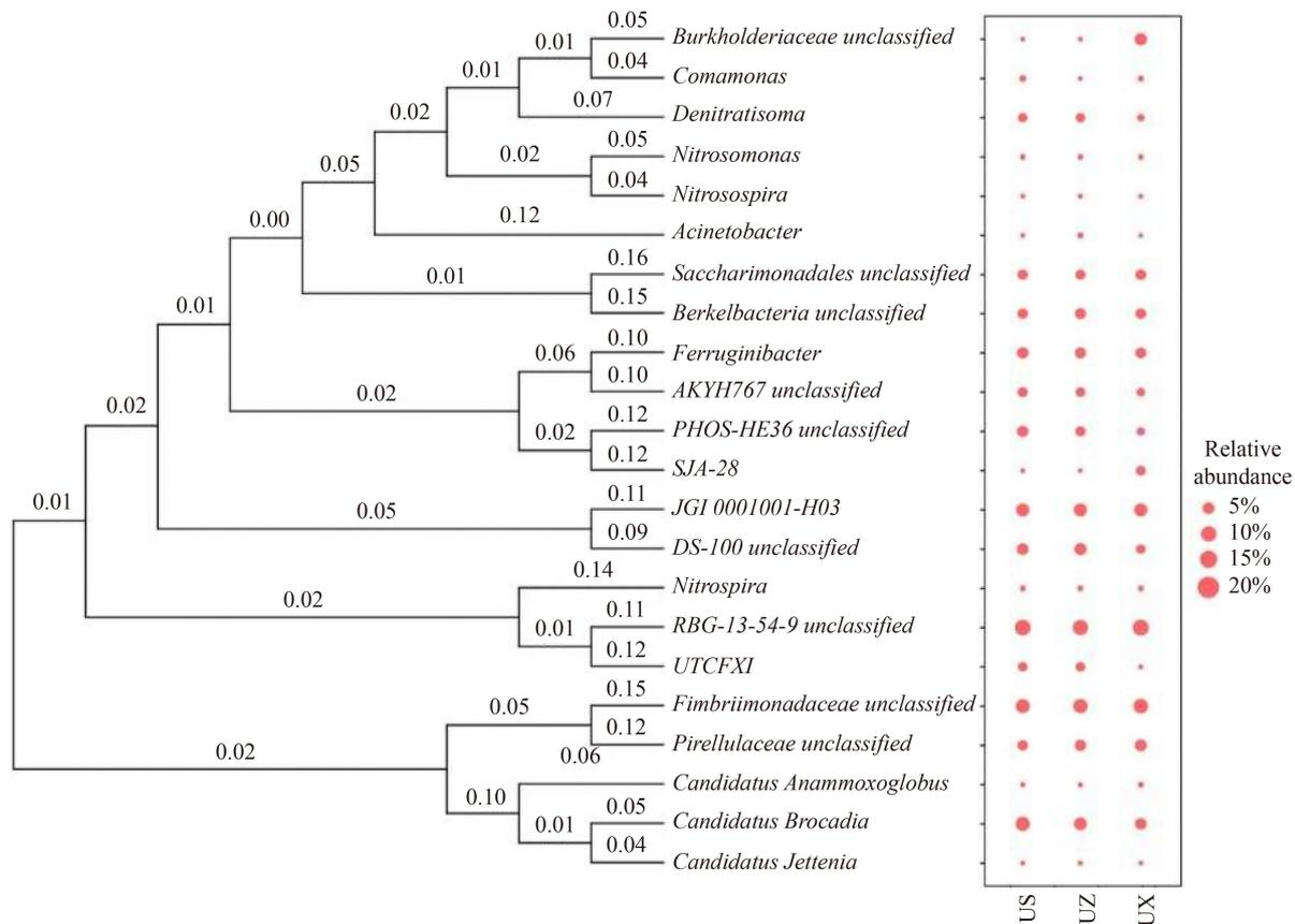
**Fig. 5** Relative abundance of major microorganisms in the Anammox-UASB system when  $HRT_{PN/A}$  was 6 h. Numbers on the branches of the phylogenetic tree indicate the branch distance. On the horizontal axis, US, UZ, and UX, respectively, indicate that the samples are taken from the upper, middle, and bottom of the UASB.
