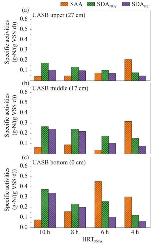
Fig. 4 Microbial activity in the Anammox-UASB: (a) UASB upper (27 cm), (b) UASB middle (17 cm), (c) UASB bottom (0 cm).
