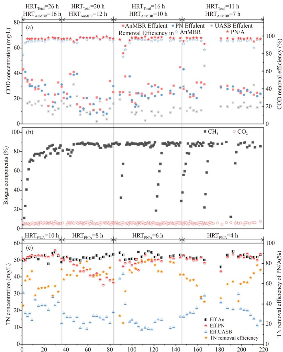
**Fig. 1** (a) COD removal performance in the AnMBR-PN/A; (b) the proportion of CH<sub>4</sub> and CO<sub>2</sub> in the biogas; (c) total nitrogen removal performance in PN/A.
