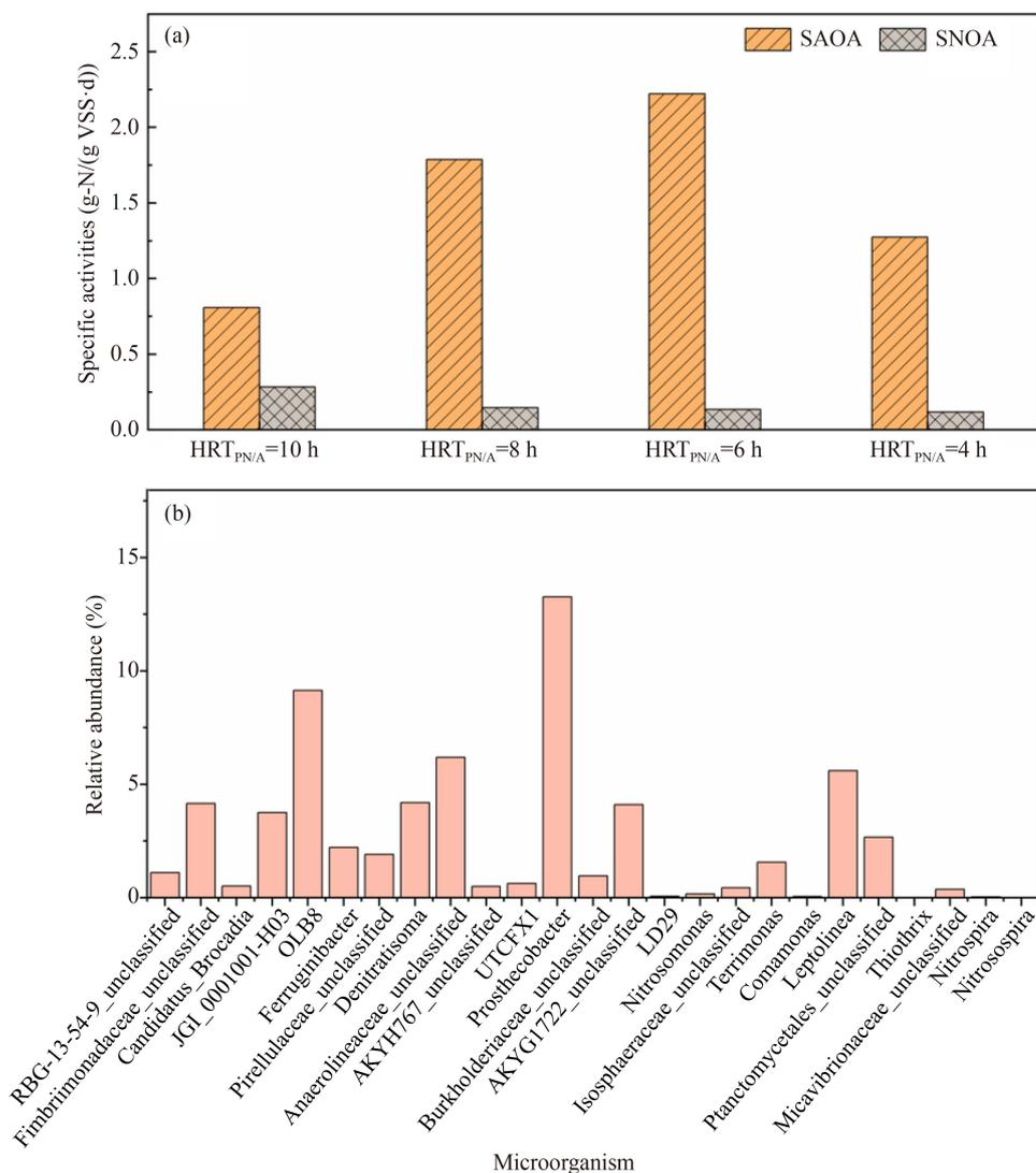
**Fig. 3** (a) Specific microbial activity of AOB and NOB in the PN-SBR; (b) relative abundance of major microorganisms in the PN-SBR when  $\text{HRT}_{\text{PN/A}}$  was 6 h.
