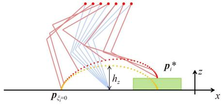
**Fig. 10** Swing trajectory based on cycloid spatial composite trajectory.
