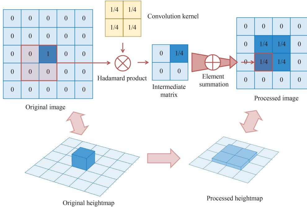
**Fig. 5** Example of image convolution in digital image processing.
