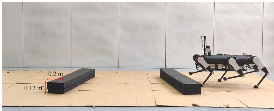
**Fig. 12** Experiment setup for footholds optimization with the hexapod robot.
