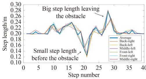
**Fig. 17** Step length with footholds optimization.
