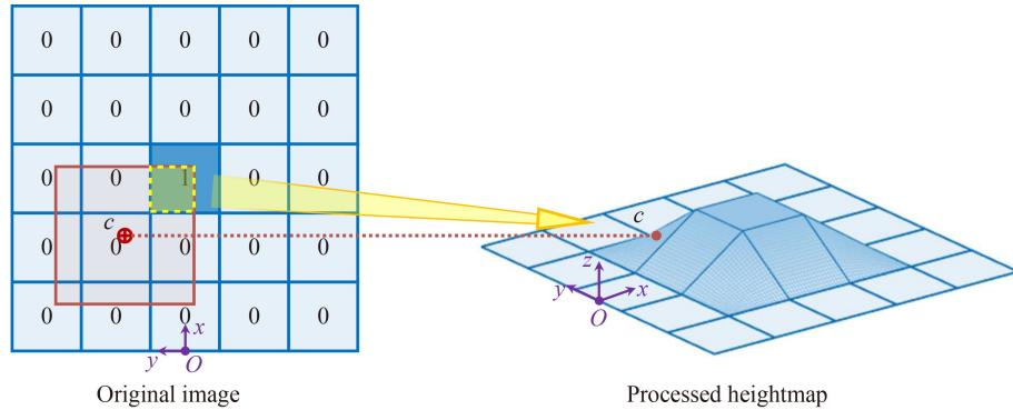
**Fig. 6** Convolution interpolation for transforming a pixel into a continuous heightmap.
