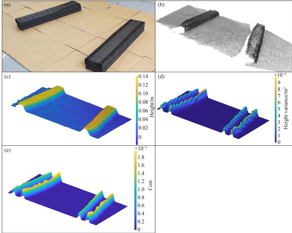
**Fig. 9** Experimental environment and the postprocessing: (a) photograph, (b) point cloud, (c) heightmap, (d) height difference map, and (e) costmap.
