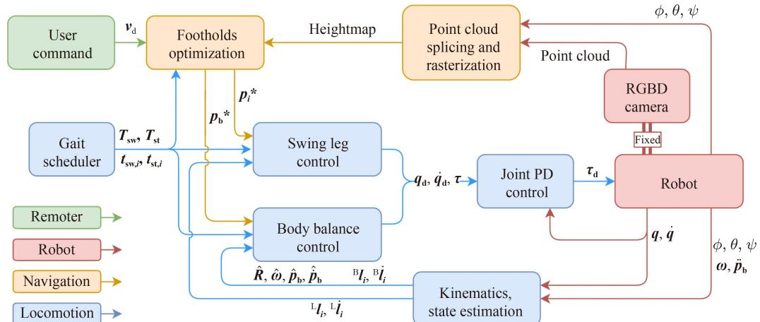
**Fig. 3** Control framework of the robot for footholds optimization.
