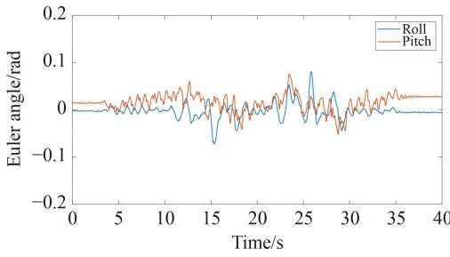
**Fig. 18** Euler angles when using foothold optimization.
