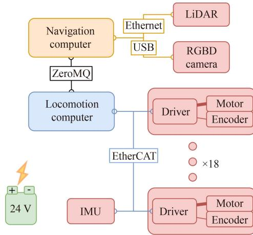
**Fig. 2** Electrical system of the robot. IMU: inertial measurement unit, RGBD: red, green, blue, depth.
