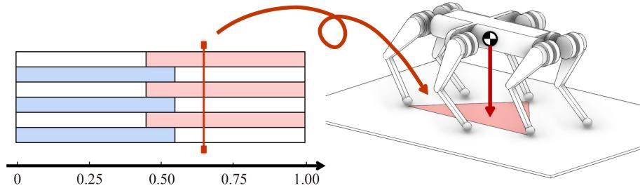
**Fig. 4** Gait scheduler and tripod-trot gait for the robot.
