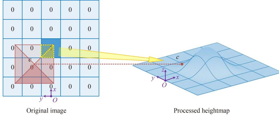
**Fig. 7** Pyramid convolution interpolation for transforming a pixel into a continuous heightmap.
