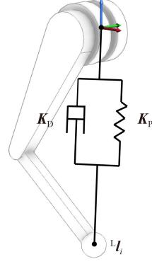
**Fig. 11** Leg virtual model of impedance control.
