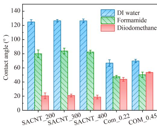
**Fig. 5** Comparison of surface wetting behavior in terms of static contact angles measured with three different liquids (i.e., DI water, formamide, and diiodomethane) among the SACNT\_200, SACNT\_300, SACNT\_400, Com\_0.22, and Com\_0.45 membranes.
