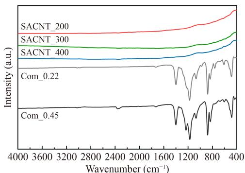
**Fig. 4** Comparison of the FTIR spectra among the SACNT\_200, SACNT\_300, SACNT\_400, Com\_0.22 PVDF, and Com\_0.45 PVDF membranes.
