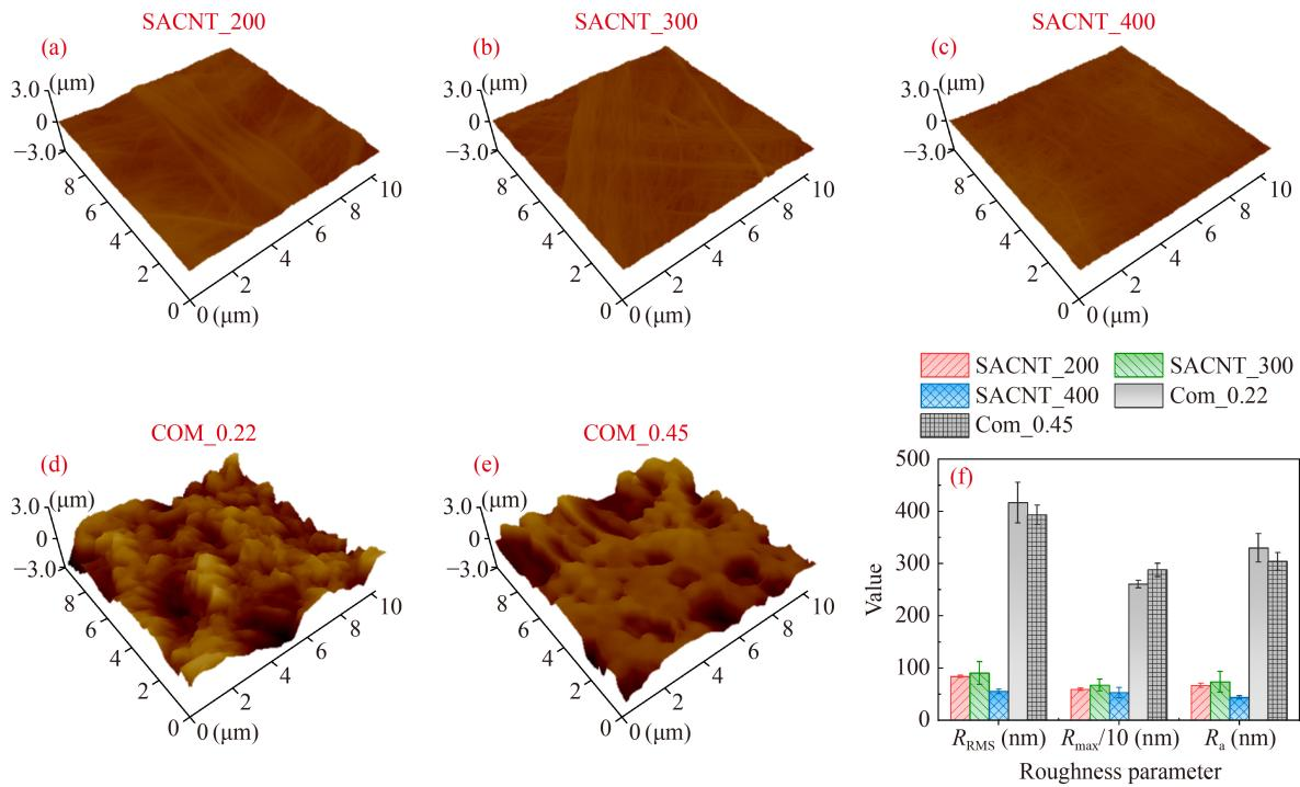
**Fig. 3** Surface morphology by AFM of the (a) SACNT\_200, (b) SACNT\_300, (c) SACNT\_400, (d) Com\_0.22, and (e) Com\_0.45 membranes. (f) Comparison in terms of three surface Roughness parameter (i.e.,  $R_{\text{RMS}}$ ,  $R_{\max}/10$ , and  $R_a$ ) among these membranes.
