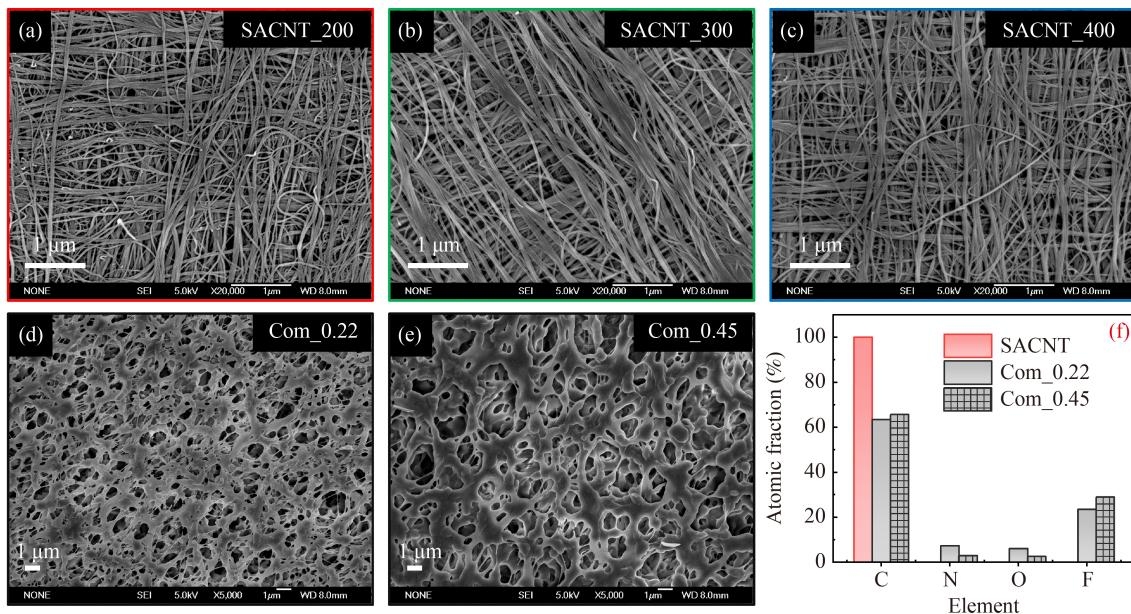
**Fig. 2** SEM top views of the (a) SACNT\_200, (b) SACNT\_300, (c) SACNT\_400, (d) Com\_0.22 PVDF, and (e) Com\_0.45 PVDF membranes. (f) Comparison of elemental compositions among the typical SACNT membrane (taking SACNT\_200 as a representative) and commercial membranes.
