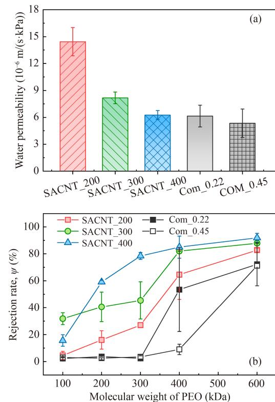
**Fig. 6** Comparison of pure water permeability and selectivity in terms of molecular weight cutoff (MWCO) among the SACNT\_200, SACNT\_300, SACNT\_400, Com\_0.22, and Com\_0.45 membranes.
