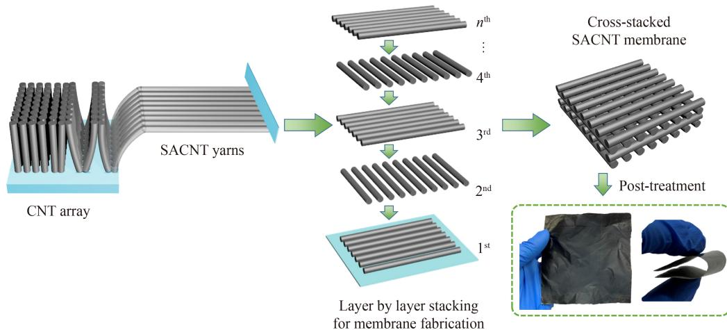
**Fig. 1** Schematic illustrating the fabrication process of the super-aligned carbon nanotube (SACNT) membrane via a layer-by-layer cross-stacking strategy. Photographs of a prepared flexible and self-supported membrane are included.
