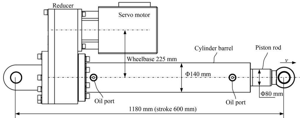
Fig. 7 Dimension diagram of electromechanical-hydraulic hybrid actuator.
