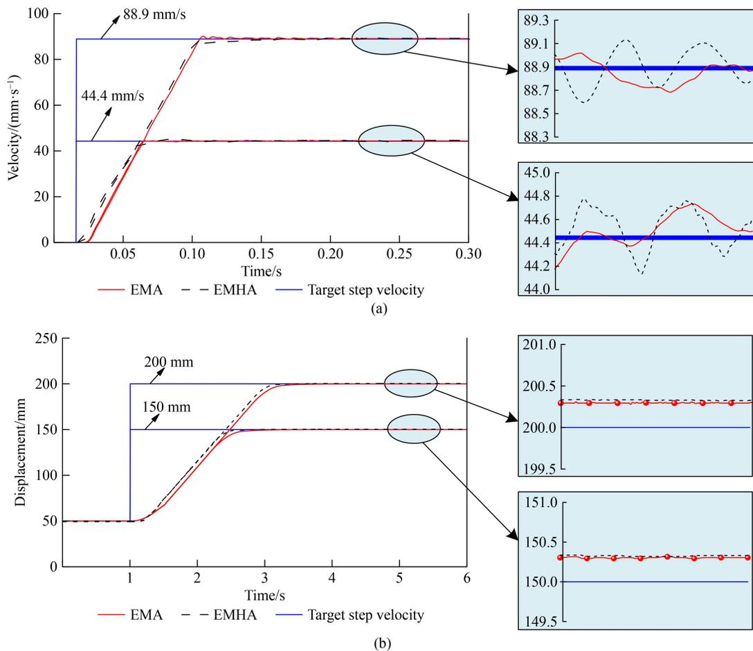
**Fig. 11** Motion control characteristic curves: (a) velocity step characteristic and (b) position step characteristic. EMA: electromechanical actuator, EMHA: electromechanical-hydraulic hybrid actuator.
