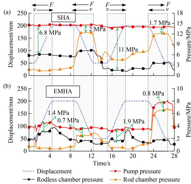
**Fig. 13** Pressure characteristic curves of actuators: (a) pressure characteristic curves of servo-hydraulic actuator (SHA) and (b) pressure characteristic curves of electromechanical-hydraulic hybrid actuator (EMHA).
