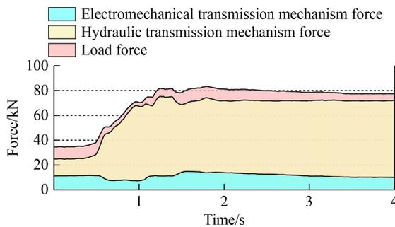
Fig. 15 Force curves of the electromechanical-hydraulic hybrid actuator transmission mechanisms.
