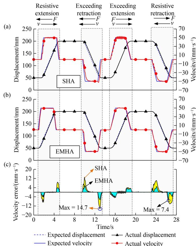
**Fig. 12** Velocity and displacement tracking characteristic curves of actuators: (a) velocity and displacement tracking characteristic curves of servo-hydraulic actuator (SHA), (b) velocity and displacement tracking characteristic curves of electromechanical-hydraulic hybrid actuator (EMHA), and (c) velocity error characteristic curves.
