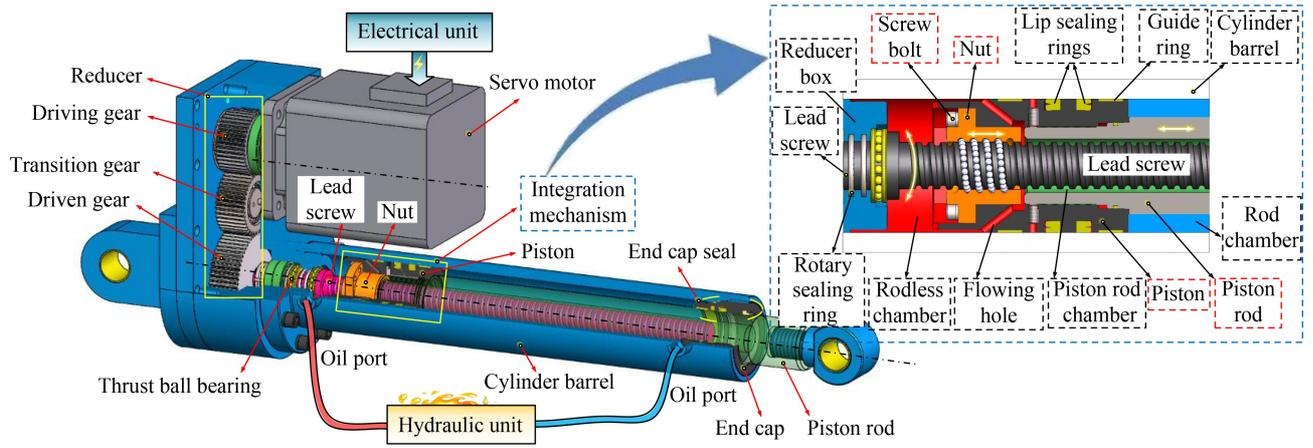
Fig. 6 Three-dimensional structure diagram of electromechanical-hydraulic hybrid actuator.
