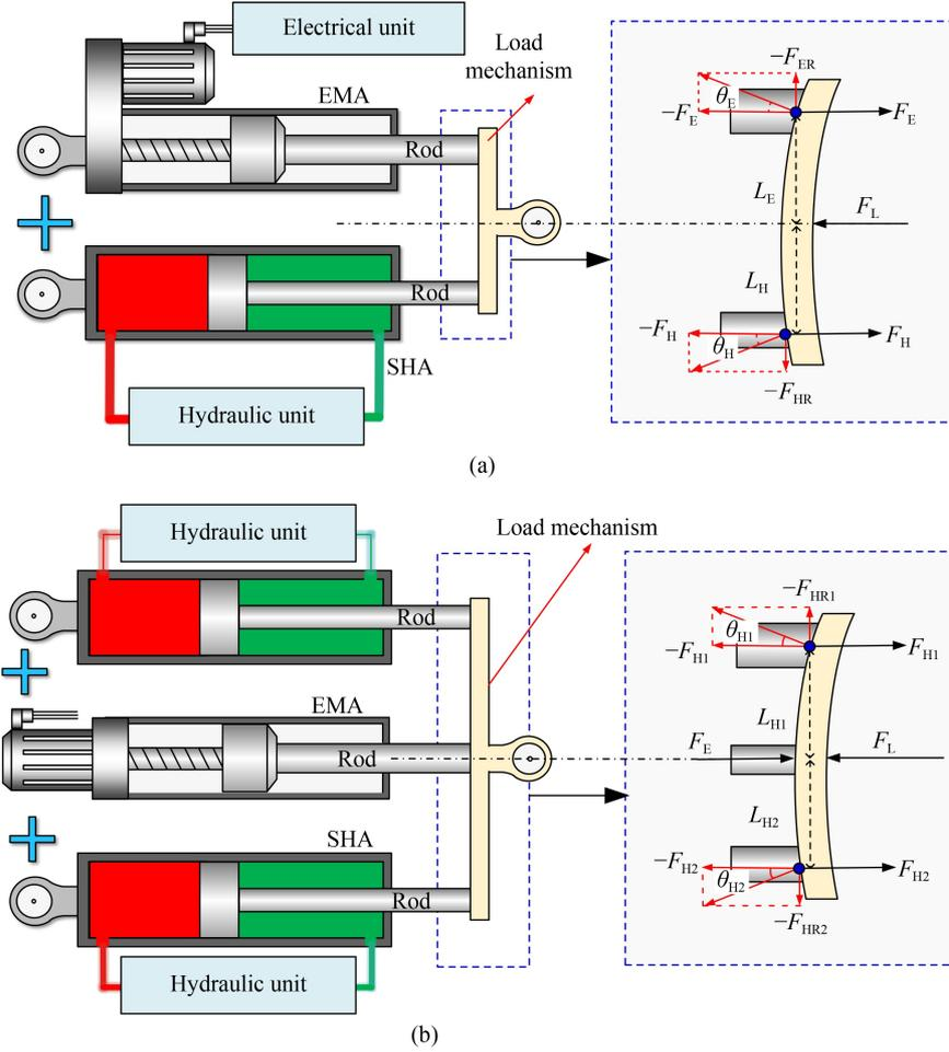
**Fig. 1** Distributed electromechanical-hydraulic hybrid linear drive system: (a) double-actuator coupling drive mechanism and (b) symmetrical coupling drive mechanism with multiple actuators. EMA: electromechanical actuator, SHA: servo-hydraulic actuator.
