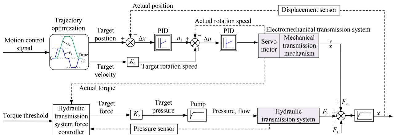
Fig. 4 Control strategy of electromechanical-hydraulic hybrid actuator.
