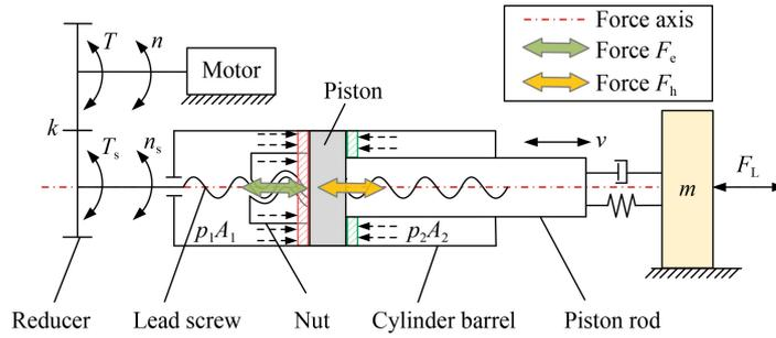
Fig. 5 Simplified structure diagram of electromechanical-hydraulic hybrid actuator.
