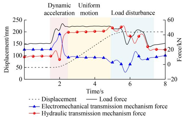
Fig. 16 Dynamic test characteristic curves of electromechanical-hydraulic hybrid actuator.
