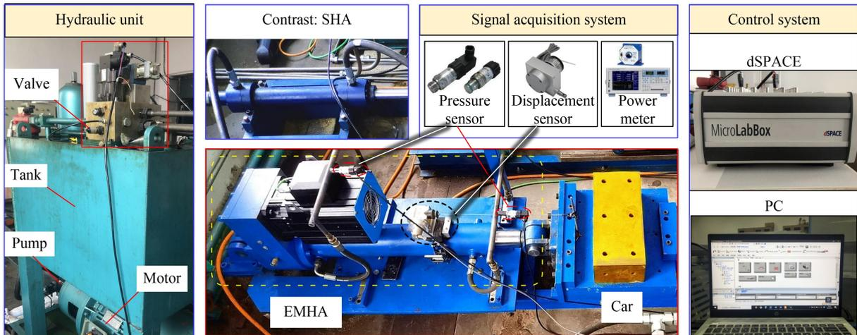
**Fig. 10** Photograph of the test platform for linear actuator. EMHA: electromechanical-hydraulic hybrid actuator, SHA: servo-hydraulic actuator.
