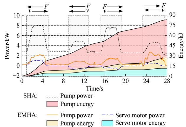
**Fig. 14** Energy consumption characteristic curves. SHA: servo-hydraulic actuator, EMHA: electromechanical-hydraulic hybrid actuator.
