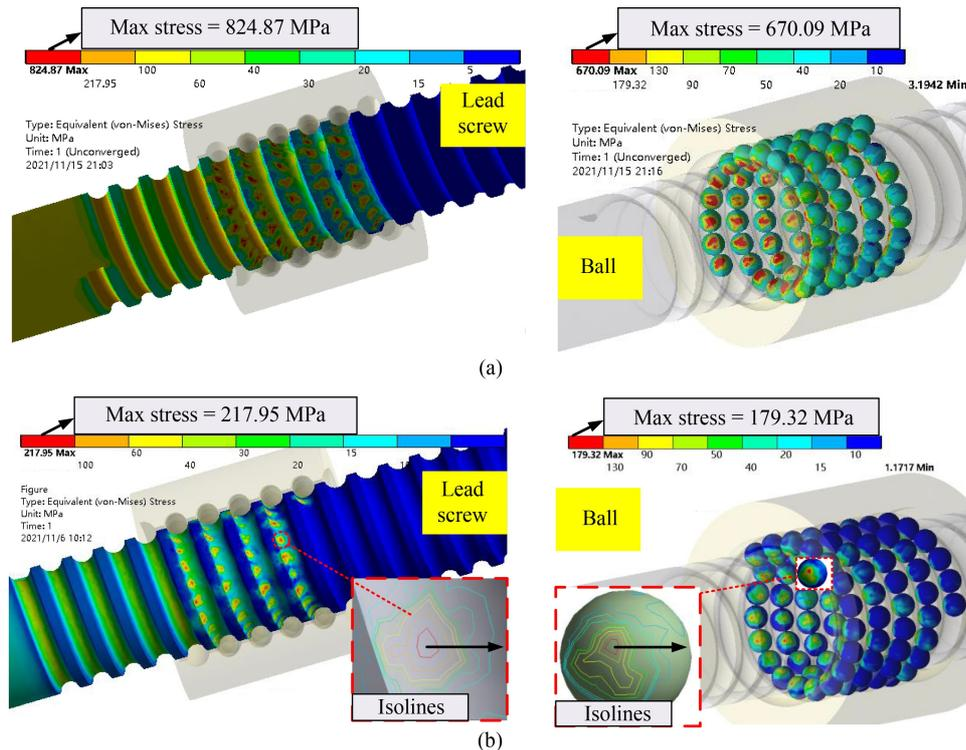
Fig. 8 Stress nephogram of the ball screw component: (a) electromechanical actuator with no hydraulic assistance and (b) electromechanical-hydraulic hybrid actuator with hydraulic assistance.
