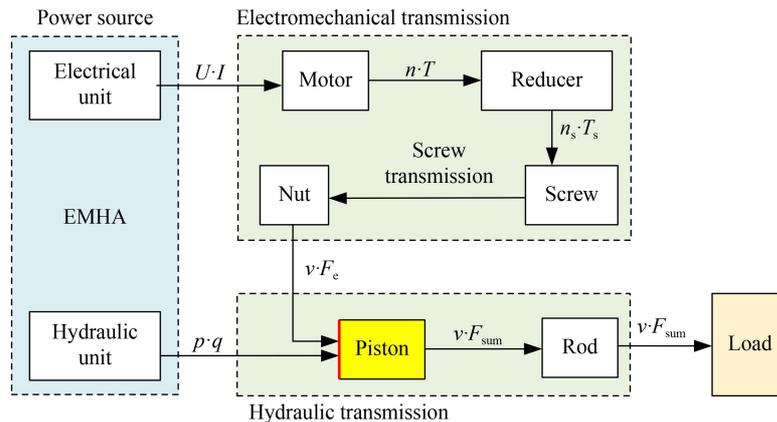
Fig. 3 Power flow diagram of electromechanical-hydraulic hybrid actuator (EMHA).
