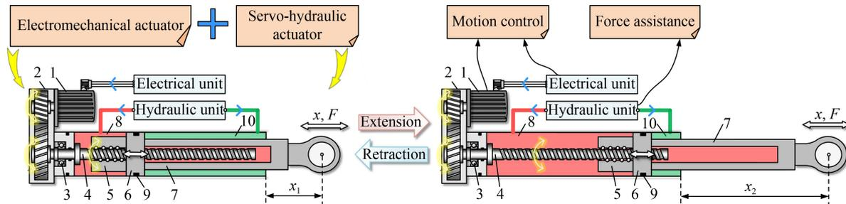
Fig. 2 Schematic diagram of electromechanical-hydraulic hybrid actuator. 1–servo motor, 2–reducer, 3–bearing, 4–lead screw, 5–nut, 6–piston, 7–piston rod, 8–rodless chamber, 9–sealing ring, 10–rod chamber.
