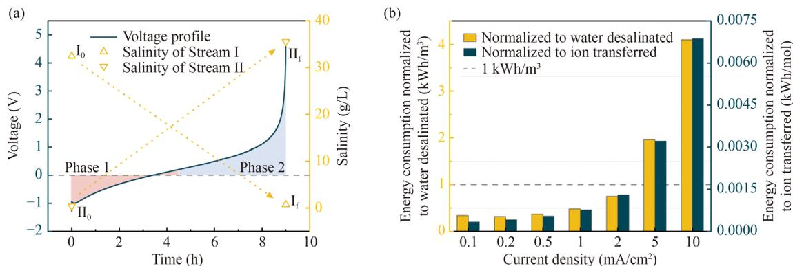
**Fig. 2** Demonstration of the SEE process with simulated seawater (0.6 mol/L NaCl) and domestic wastewater (0.01 mol/L NaCl). (a) Voltage profile and salinity change of the two streams in a typical SEE operation and (b) energy consumption of the SEE process at different current densities. In (a) the blue curve represents the measured voltage over time with the shaded portions above and below representing the energy generation and consumption phases.
