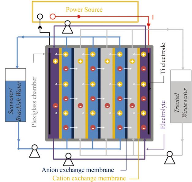
**Fig. 1** Operation of a salinity exchange electro dialysis (SEE) system.
