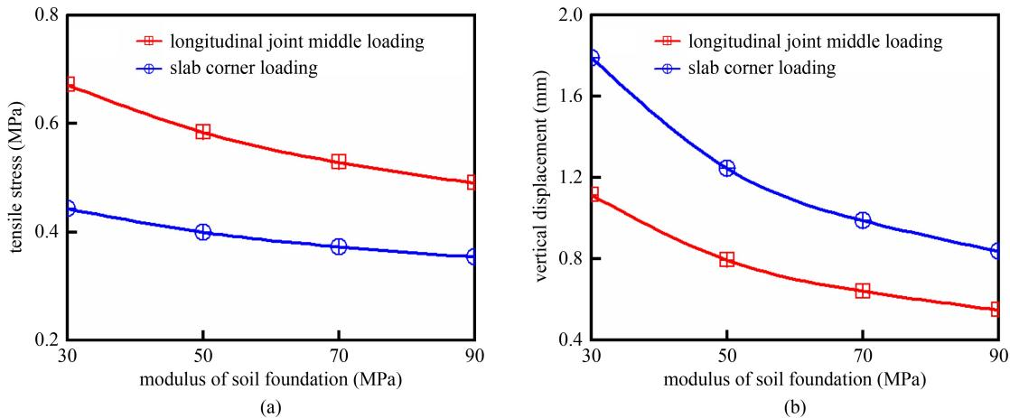
**Fig. 16** Mechanical response of plastic pavement under different soil foundation modulus: (a) maximum tensile stress; (b) vertical displacement.
