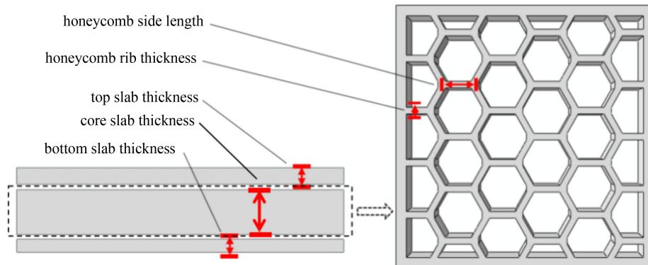
**Fig. 3** Schematic diagram of the honeycomb structure pavement slab.
