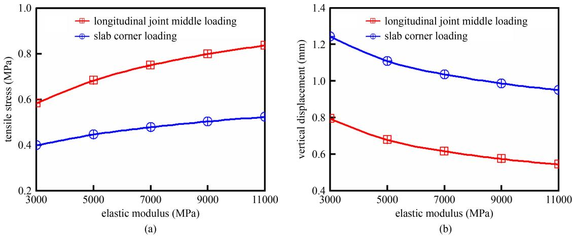
Fig. 13 Mechanical response of plastic pavement under different plastic material modulus: (a) maximum tensile stress; (b) vertical displacement.
