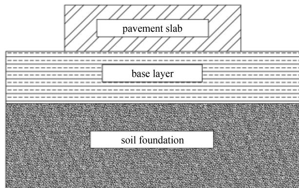
Fig. 1 Schematic diagram of plastic pavement structure model.
