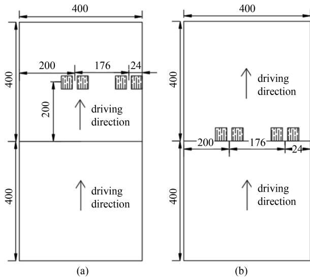
**Fig. 2** Loading acting position (unit: mm): (a) middle of longitudinal joint; (b) slab corner.
