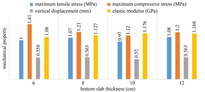
**Fig. 5** Mechanical properties of plastic pavement slabs under different bottom slab thickness.
