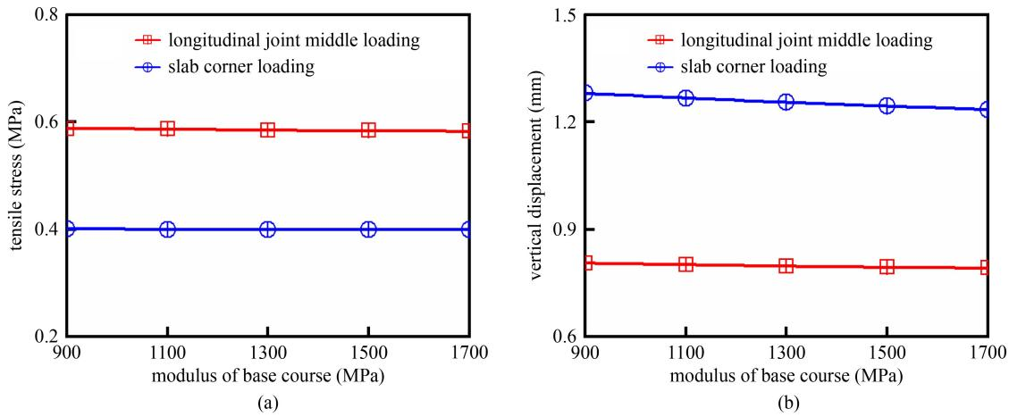
**Fig. 15** Mechanical response of plastic pavement under different base layer modulus: (a) maximum tensile stress; (b) vertical displacement.
