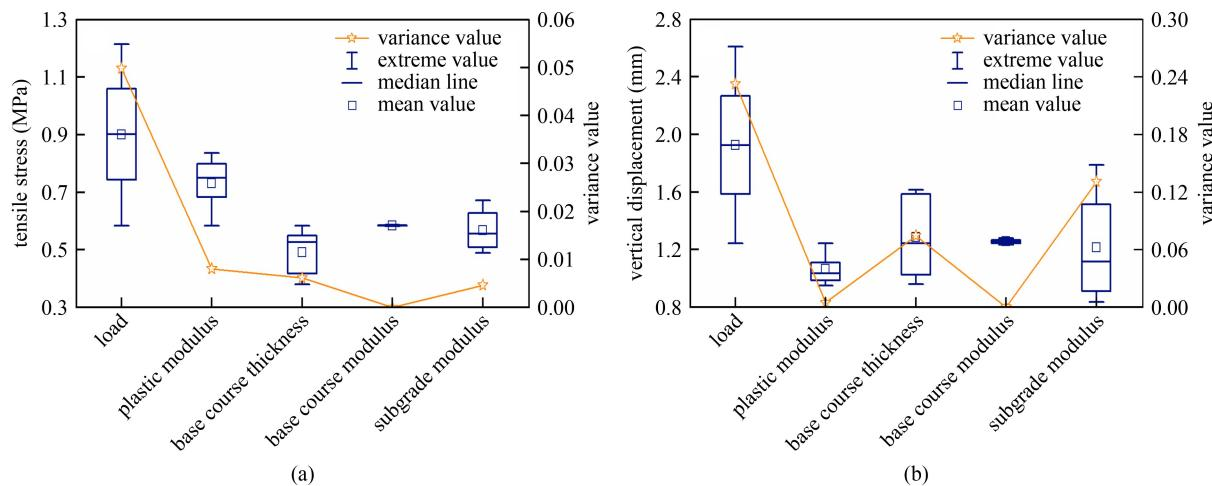
Fig. 17 Influence degree of various factors on: (a) tensile stress; (b) vertical displacement.
