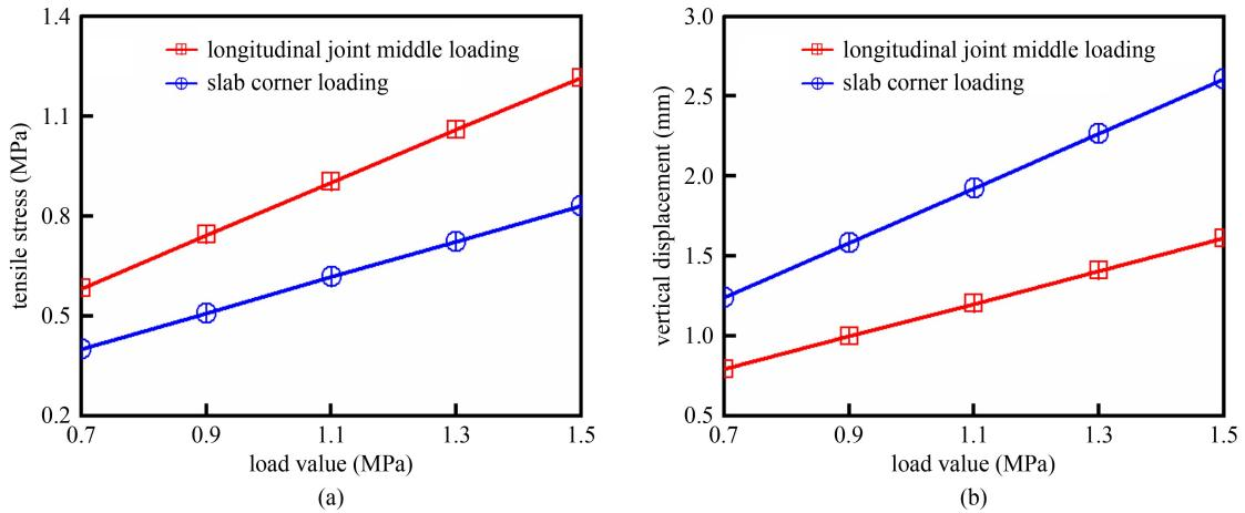
**Fig. 12** Mechanical response of plastic pavement under different loads: (a) maximum tensile stress; (b) vertical displacement.
