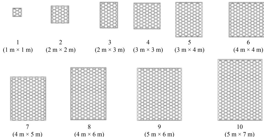
**Fig. 9** Dimension model of plastic pavement slab.
