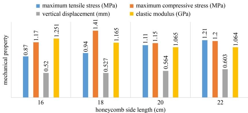
**Fig. 7** Mechanical properties of plastic pavement slabs under different honeycomb side length.
