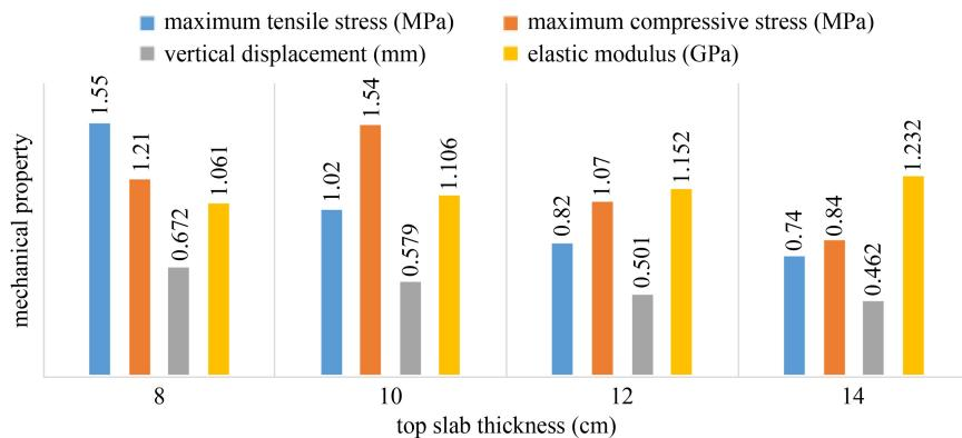
**Fig. 6** Mechanical properties of plastic pavement slabs under different top slab thickness.
