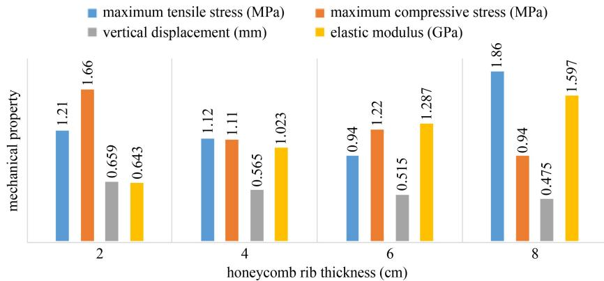
**Fig. 8** Mechanical properties of plastic pavement slabs under different honeycomb rib thickness.
