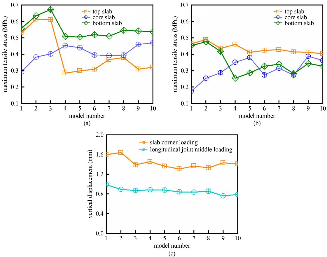
**Fig. 10** Maximum tensile stress: (a) under longitudinal joint middle loading; (b) under corner loading; and (c) vertical displacement of the honeycomb structure with different plain view size.
