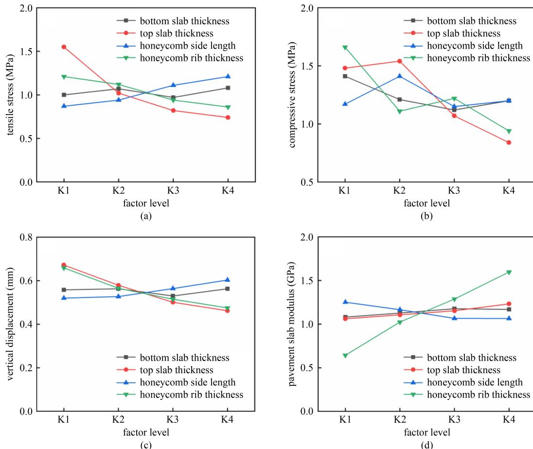
**Fig. 4** Influence of geometric dimensions on: (a) maximum tensile stress; (b) maximum compressive stress; (c) vertical displacement; (d) pavement slab elastic modulus of honeycomb structure.
