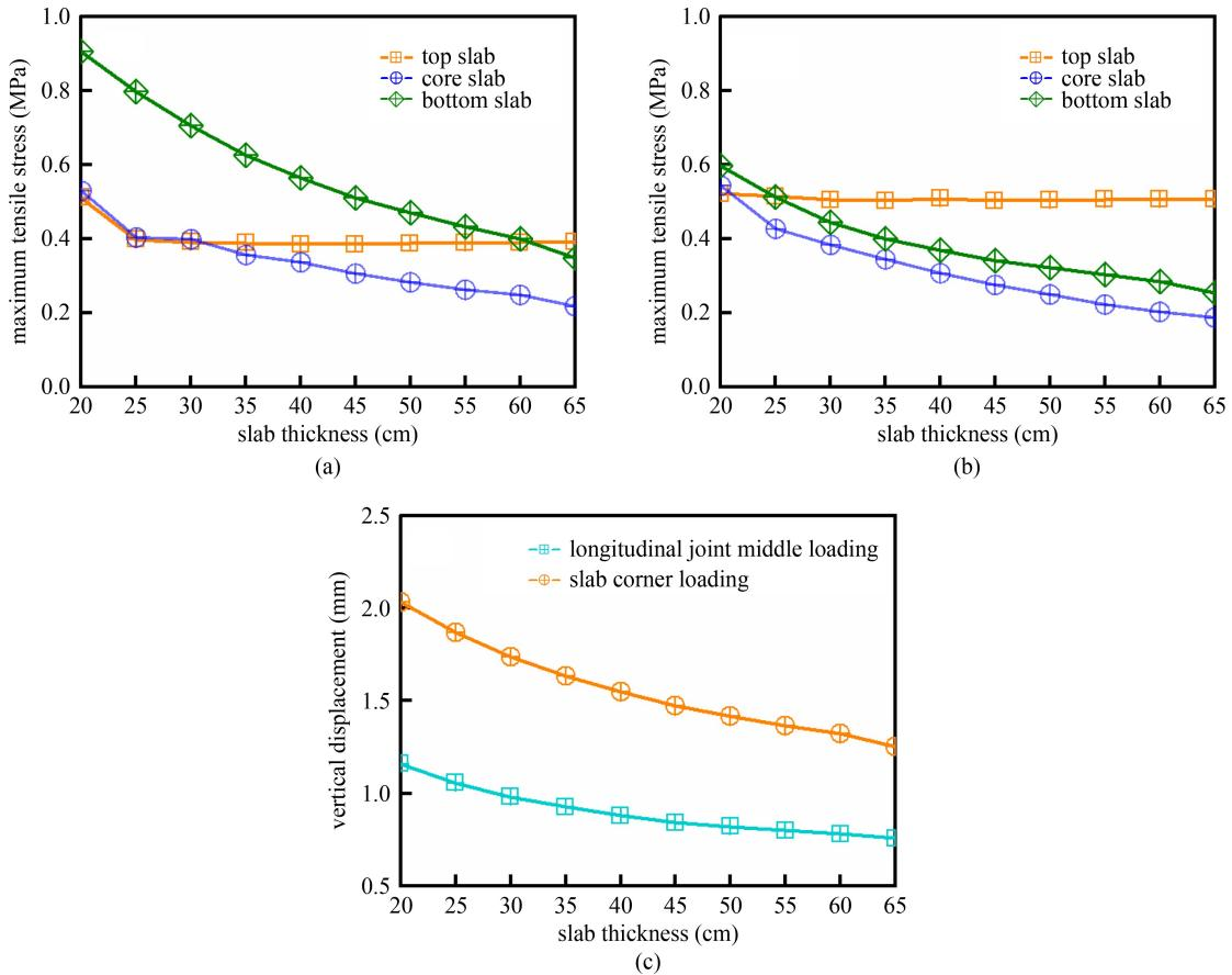
**Fig. 11** Maximum tensile stress: (a) under longitudinal joint middle loading; (b) under corner loading; and (c) vertical displacement of the honeycomb structure with different slab thickness.
