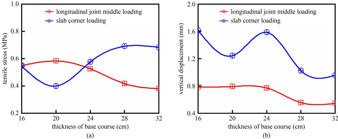
Fig. 14 Mechanical response of plastic pavement under different base layer thickness: (a) maximum tensile stress; (b) vertical displacement.
