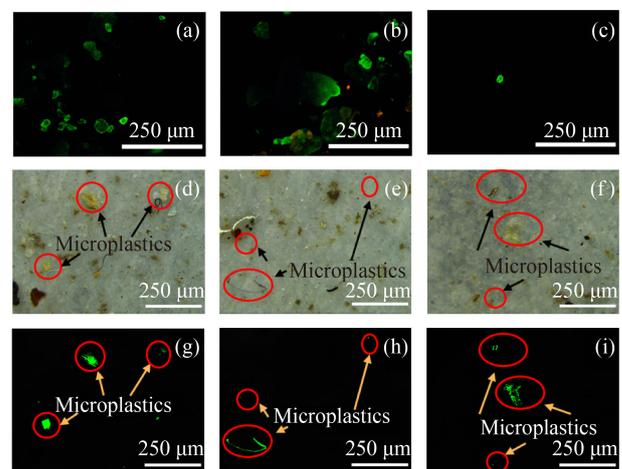
**Fig. 2** The microscope images of MPs were stained with NR (a)–(c). The microscope images of MPs in the bright field after staining (d)–(f). The microscope images of the stained MPs in the dark field after processing with ImageJ software (g)–(i).
