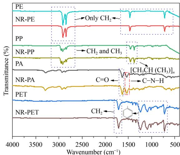
**Fig. 3** ATR FT-IR spectra of PE, PP, PA, and PET before and after stained by Nile Red solution.
