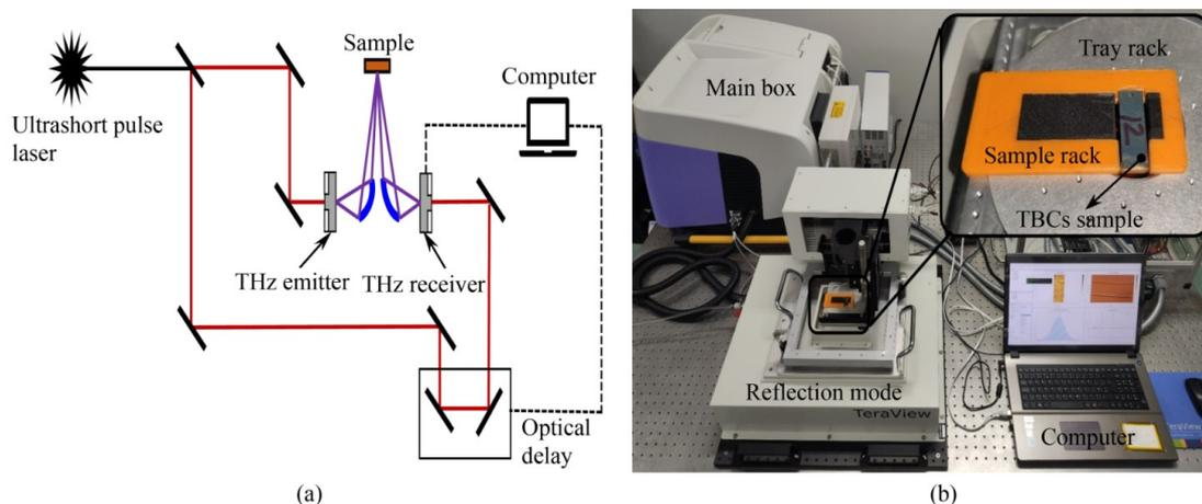
**Fig. 6** TeraPulse 4000 system: (a) system structure diagram and (b) actual system.
