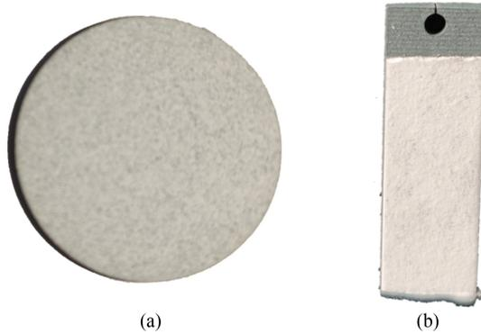
**Fig. 7** Thermal barrier coating samples: (a) round sample and (b) rectangular sample.
