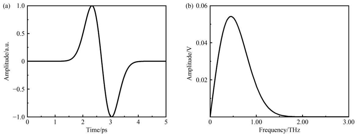
Fig. 2 Terahertz incident signal in simulation: (a) time-domain pulse and (b) its frequency spectrum.
