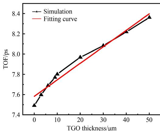
**Fig. 5** Linear relationship between the time of flight (TOF) and the thermally grown oxide (TGO) thickness.
