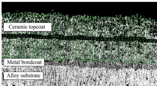
**Fig. 9** Scanning electron microscope measurement of ceramic thickness in thermally barrier coatings without thermal cycling.
