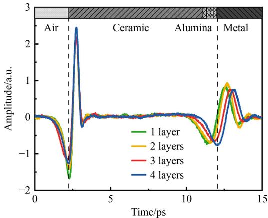
**Fig. 8** Terahertz time-domain signals of thermal barrier coatings for different layer alumina.
