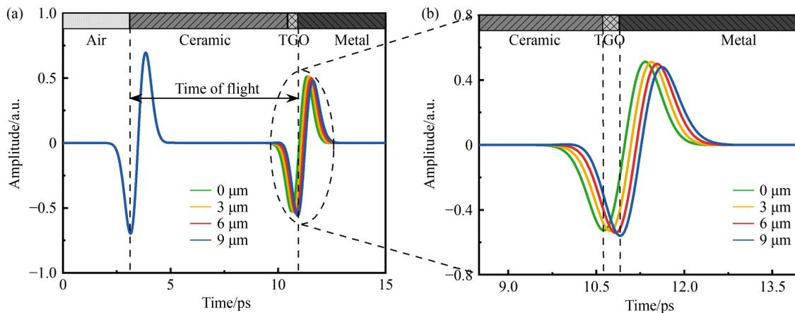
**Fig. 4** Terahertz propagation waveform for the actual thickness range of the thermally grown oxide (TGO): (a) terahertz propagation waveform and (b) its local waveform.
