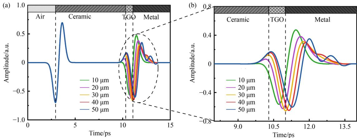
Fig. 3 Terahertz propagation waveform with different thicknesses of the thermally grown oxide (TGO): (a) terahertz propagation waveform and (b) its local waveform.
