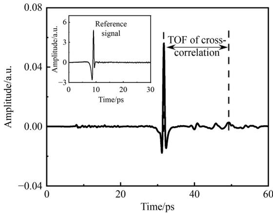
**Fig. 13** Cross-correlation function wave between the reference signal and terahertz signal. TOF: time of flight.
