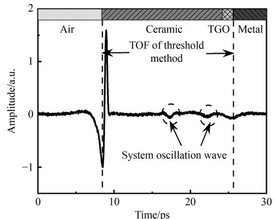
**Fig. 11** Terahertz signal interfered by environmental noise and system oscillation. TGO: thermally grown oxide; TOF: time of flight.
