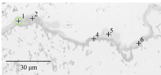
**Fig. 10** Thermally grown oxide morphology after 60 h heating times.
