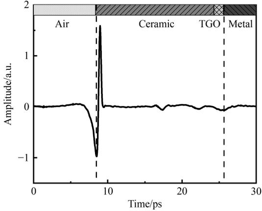
**Fig. 12** Denoised terahertz signal used wavelet soft threshold method. TGO: thermally grown oxide.
