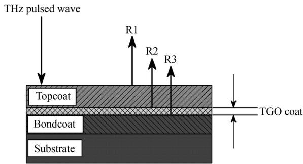
**Fig. 1** Typical thermal barrier coating system with thermally grown oxide (TGO).
