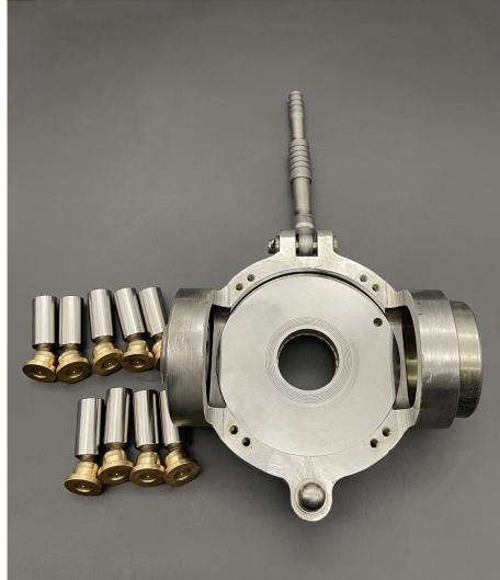
**Fig. 13** Assembly of the swash plate with texture design.
