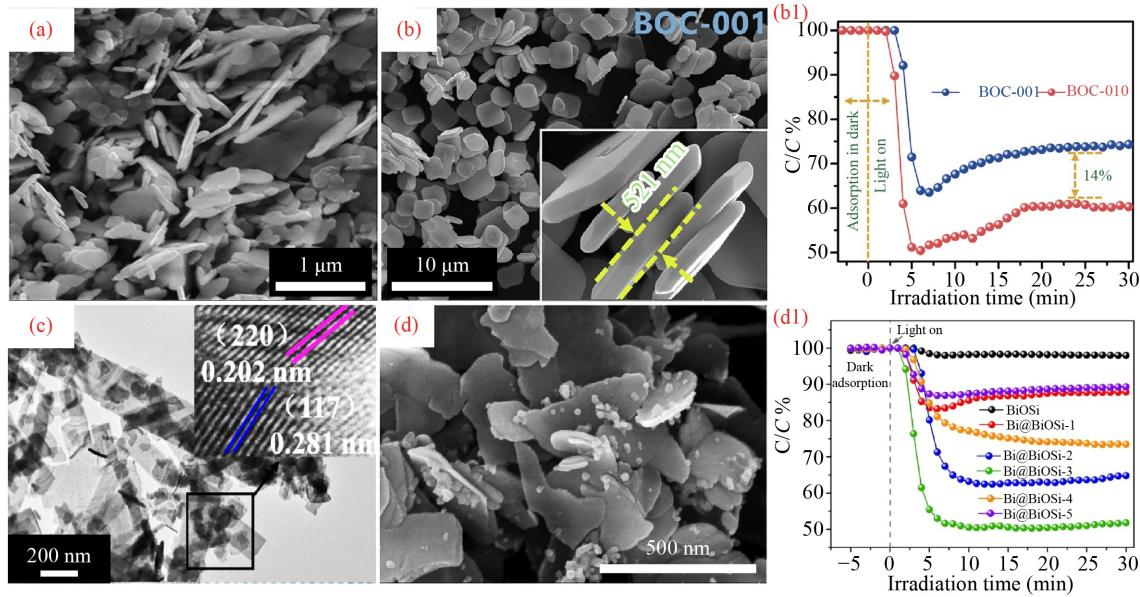
**Fig. 5** 2D Bi-based materials with plate shapes on photocatalytic NO degradation: BiOCl (a, (Xie et al., 2020), b, (Li et al., 2019a)), Bi<sub>24</sub>O<sub>31</sub>Br<sub>10</sub>/Bi<sub>3</sub>O<sub>4</sub>Br (c, (Li et al., 2020b)) and Bi/Bi<sub>2</sub>O<sub>2</sub>SiO<sub>3</sub> (d, (Li et al., 2019d)). The figures are all copyrighted from Elsevier Publishing Group.
