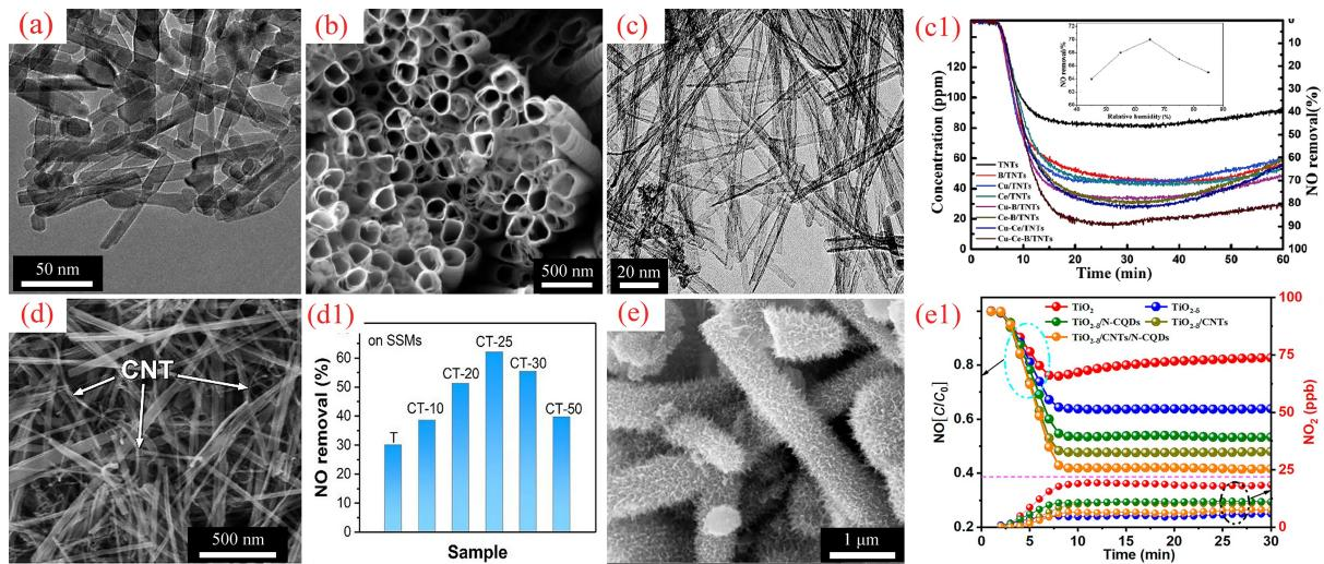
**Fig. 1** 1D  $\text{TiO}_2$  material on photocatalytic NO degradation: nanorod (a, (Habran et al., 2018)), nanotube (b, (Martin et al., 2017), c, (Li et al., 2015)), nanoparticles on C nanotubes (d, (Xiao et al., 2019)) and coral (e, (Ou et al., 2021)). The figures are copyrighted from Taylor & Francis Publishing Group (a), Elsevier Publishing Group (b), Royal Society of Chemistry Publishing Group (c) and American Chemical Society Publishing Group (d, e).
