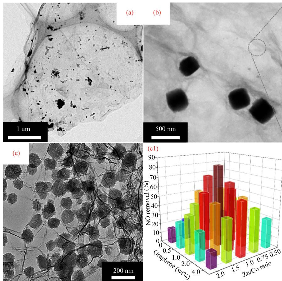
**Fig. 3** 2D GO-based materials loaded with different shapes on photocatalytic NO degradation: nanoparticles (a, (Feng et al., 2020)), cubes (b, (Hu et al., 2018)) and rhombic dodecahedron (c, (Xiao et al., 2018)). The figures are copyrighted from Royal Society of Chemistry Publishing Group (a) and Elsevier Publishing Group (b, c).
