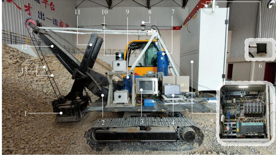
1-Dipper; 2-Crowd machinery; 3-Data acquisition system; 4-Industrial control computer; 5-Electronic control cabinet; 6-IMU; 7-Rotation machinery; 8-GNSS; 9-Hoist machinery; 10-LiDAR; 11-Dipper handle; 12-Boom; 13-Hoist rope
