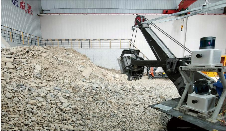
Fig. 3 3D point cloud acquisition device composed of two RS-Ruby Lite 80 laser-beam LiDARs.
