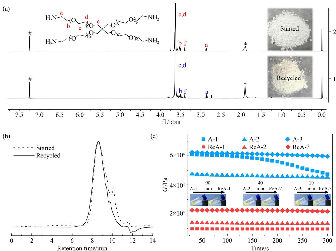
**Fig. 5** (a) Proton NMR for started and recycled 4-PEG amine in  $\text{CDCl}_3$ ; (b) GPC for started and recycled 4-PEG amine in DMF; (c) Storage modulus ( $G'$ ) and loss modulus ( $G''$ ) for ReA-1, -2, -3 after the swelling in the mode of time scan. Inset photos: regeneration of materials by using recycled 4-PEG amine in acetonitrile.
