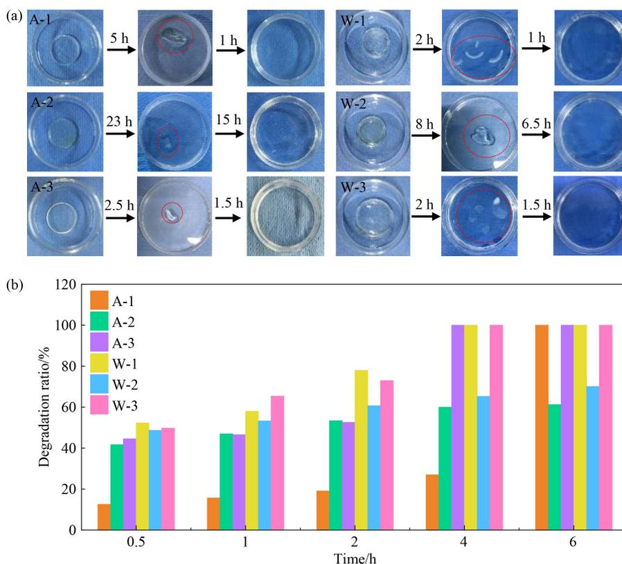
**Fig. 4** (a) Degradation of all materials by EDA (Initial status of materials (left dishes); residue of materials after degradation for a certain amount of time (middle dishes); clear solutions after complete degradation (right dishes)); (b) Kinetics of degradation for all materials in EDA through measuring weight.
