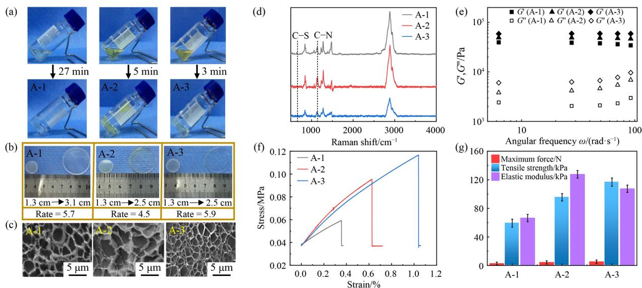
**Fig. 2** (a) Formation of A-1, -2, -3 in acetonitrile; (b) Swelling properties for A-1, -2, -3 in water, size changes and swelling ratios; (c) SEM images for A-1, -2, -3.  $M = 15$  k; (d) Raman spectra for A-1, -2, -3; (e) Storage modulus ( $G'$ ) and loss modulus ( $G''$ ) for swelled A-1, -2, -3; (f) Stress-strain tension test for swelled A-1, -2, -3; (g) Maximum force, tensile strength and elastic modulus test for swelled A-1, -2, -3.
