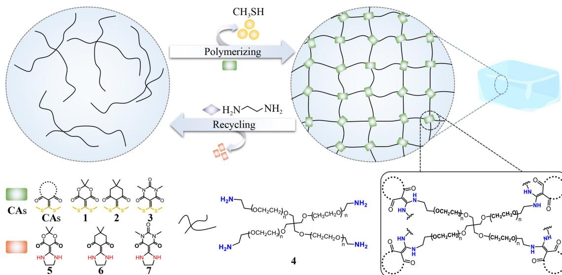
**Fig. 1** Recycling of soft materials through “amine–thiol coupling and amine–amine decoupling” reactions: materials of synthesis through the reactions between CAs 1, 2, 3 and 4-PEG amine 4 with releasing methyl mercaptan ( $\text{CH}_3\text{SH}$ ); EDA-induced decoupling to release the original amine partner 4 and five-membered ring product 5, 6, 7. The recyclable monomer was employed again to regenerate soft materials.
