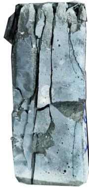
**Fig. 3** Failure pattern of the intact sample under uniaxial compression.
