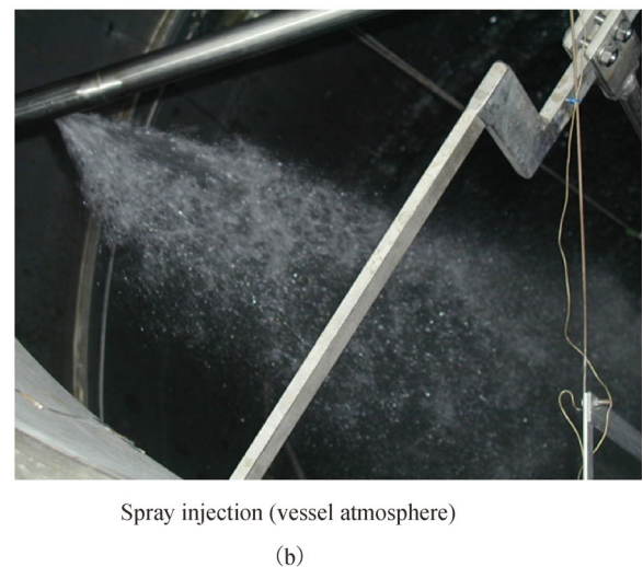
Fig. 11 Water-pool thermal stratification and spray induced mixing.
