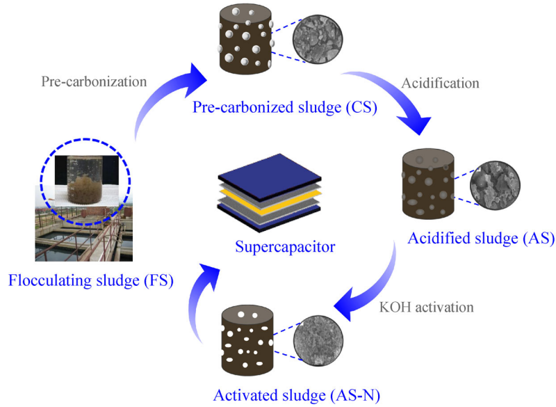
Fig. 1 Schematic procedure for the fabrication of porous electrode material from floc sludge.
