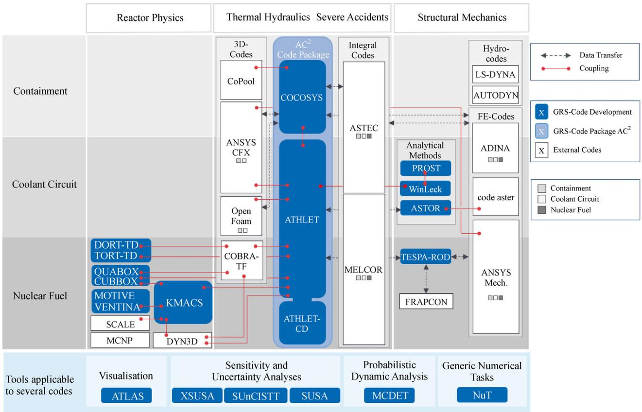
Fig. 1 The current status of the nuclear simulation chain of GRS (adapted with permission from Ref. [54]).
