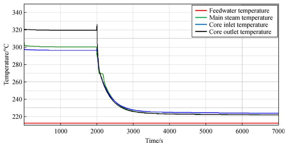
Fig. 5 Temperature evolution for a partial pump trip with scram (modified from Ref. [68]).
