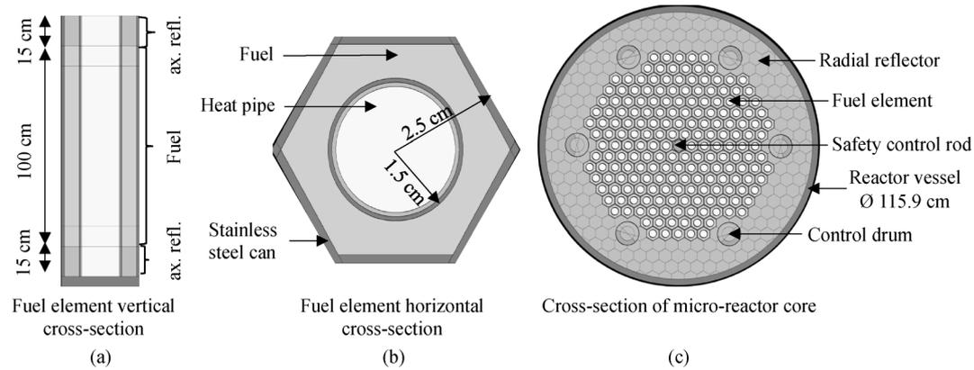
**Fig. 2** The HPMR core consisting of 192 hexagonal fuel elements surrounded by six control rod drums.
