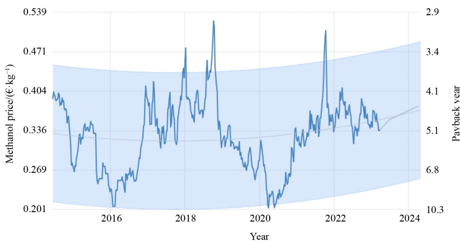
Fig. 6 The methanol price tendency in the past decade and estimated payback years.
