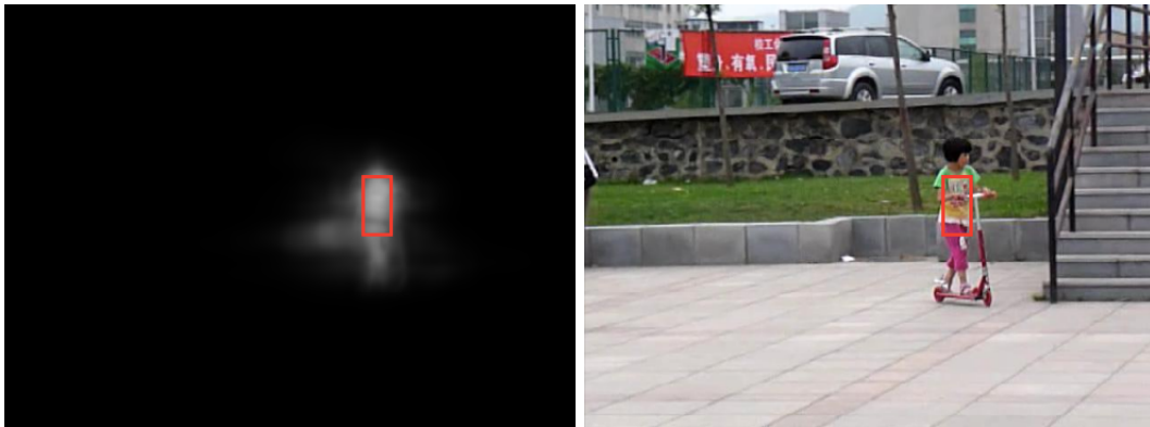
Figure 3: Left: Output of the mask with red Minimum Enclosing Rectangle. Right: The output in the frame.
