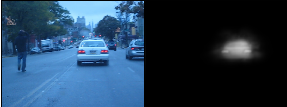
Figure 2: Left: The car in the frame to be tracked. Right: The output of LGM module with referring expression the white car in the middle .
