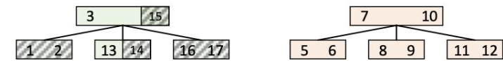
(a) The way skip works. After searching entry 3 and 13 of the left tree, we would know there are no entries smaller than 5 or larger than 12. The entries shaded can be dropped without validation.
