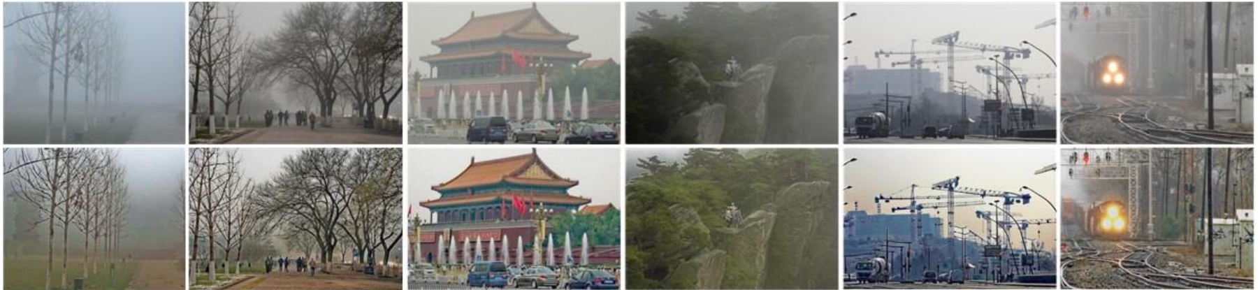
Real-world hazy images (top) and corresponding visibility restoration results (bottom) using our proposed unified variational model
