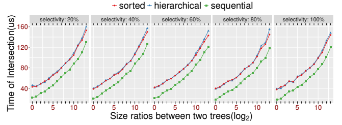
Fig. 3: Intersection time on k -ary search tree via three traversal algorithms for different size ratios and selectivities, fixing the smaller size to 1024.
