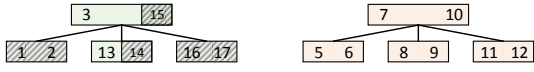
(a) The way skip works. After searching entry 3 and 13 of the left tree, we would know there are no entries smaller than 5 or larger than 12. The entries shaded can be dropped without validation.
