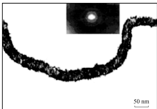
Fig. 1 TEM images and SAED of Pt-CNT The ratio of Pt to CNT is 0.1875 mmol/g
