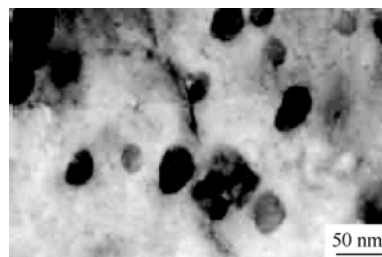
Fig. 4 FBA/PMMA particles dispersed in PA6 matrix
