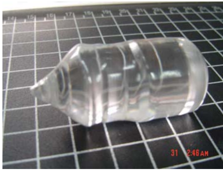
Fig. 1 The SrWO 4 single crystal grown along a -axis
