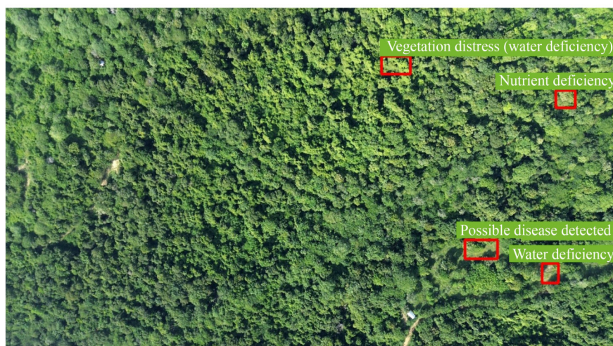
Fig. 3 Drone-based vegetation stress analysis. The drone image was captured in a remote farming region near the Caribbean coast of Colombia. Red boxes indicate potential vegetation stress due to water deficiency or disease, detected using color segmentation and edge detection ML models. Original bounding box labels were too small to read and have been relabeled for clarity.
