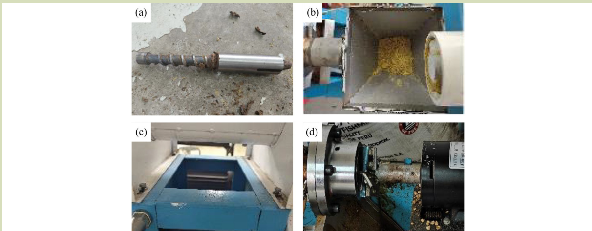
Fig. 8 The picture of puffing machine fault phenomenon. (a) Cavity blockage; (b) inlet clogged; (c) screw loosening; (d) cutter wear.
