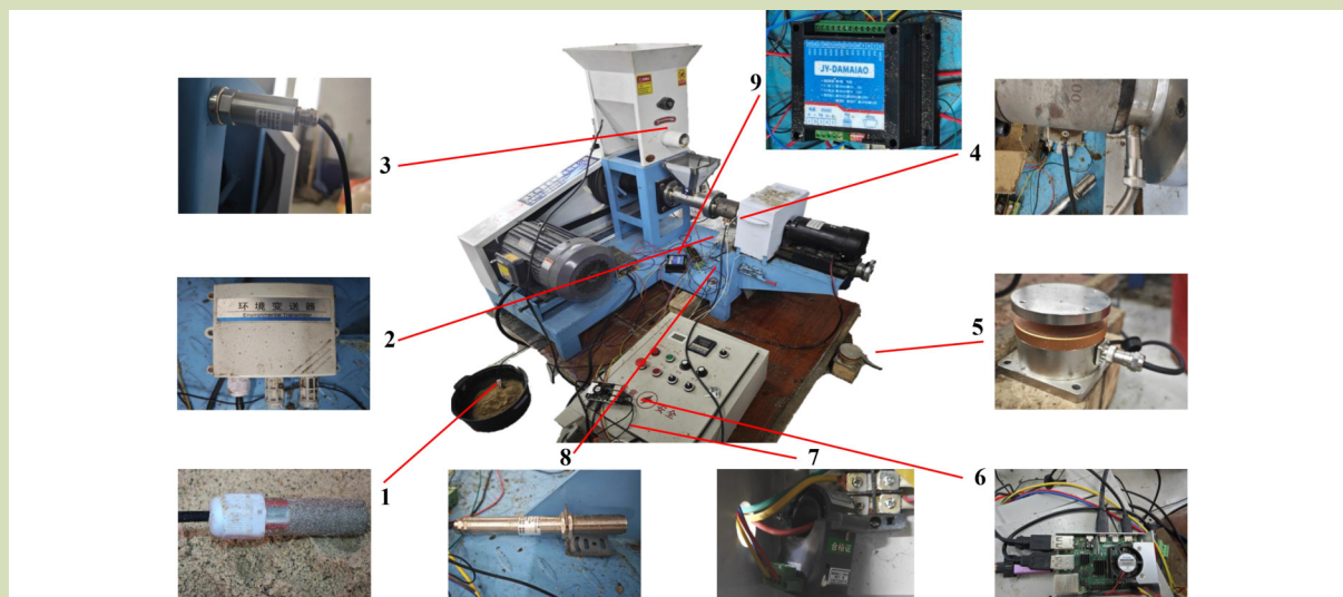
Fig. 1 Diagram of the installation of components and measuring instruments used in puffing machine. 1, Feed temperature and humidity sensor; 2, ambient temperature and humidity sensor; 3, vibration sensor; 4, temperature sensor; 5, weighing sensor; 6, Raspberry Pi data processor; 7, current sensor; and 8, noise sensor.
