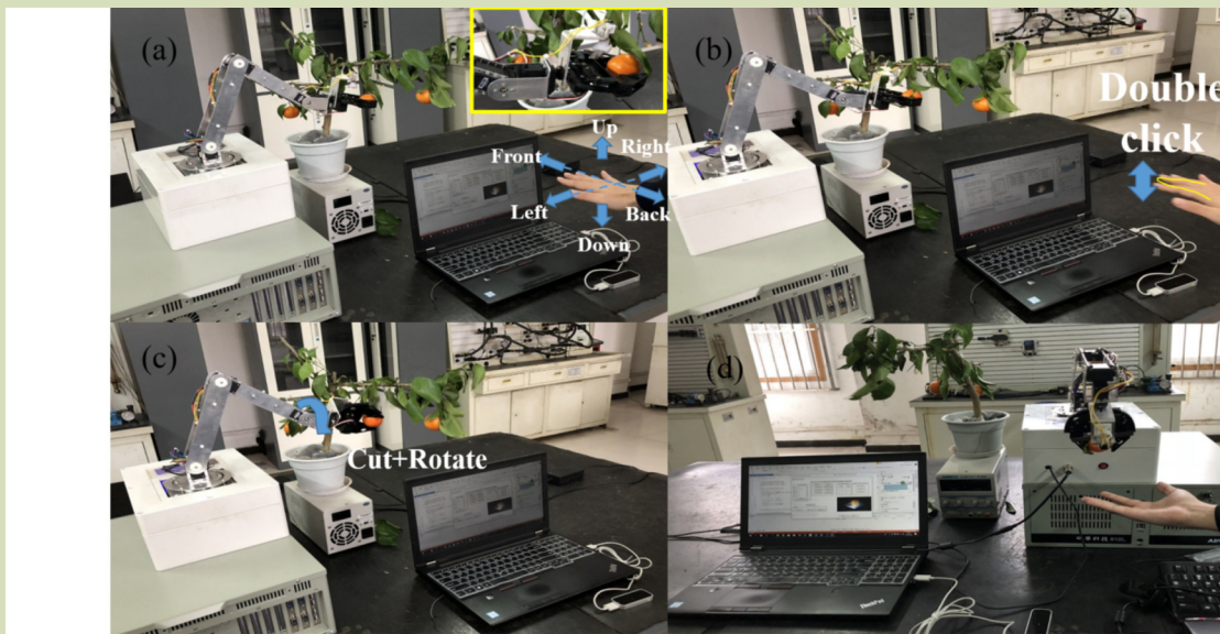
Fig. 15 Picking process of the robot. (a) Toward-target by motion-sensing; (b) picking by double click gesture; (c) automatic picking; (d) automatic unloading.
