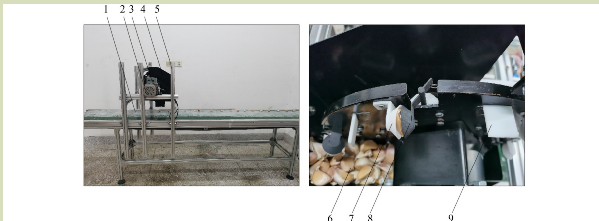
Fig. 15 Bench validation test: 1, conveyor belt; 2, motor; 3, motor governor; 4, seed-metering device; 5, mounting rack; 6, seed loading chamber; 7, seed-collection spoon; 8, pickup finger; and 9, seed-distribution plate.
