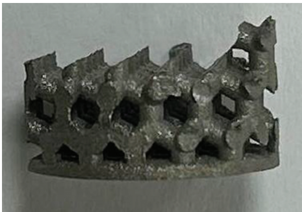
Figure 9. Side view of specimen fracture shows the fracture on the strut node with 45°
